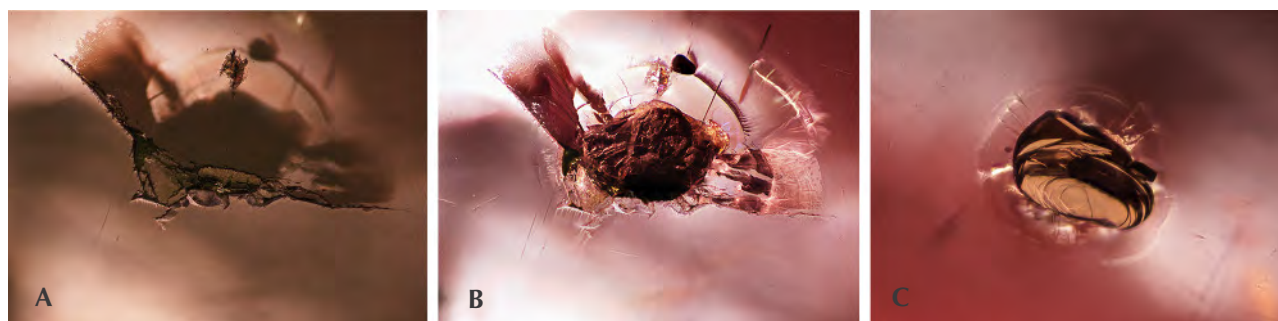
Figure 7. A: This graphite crystal with tension halo is shown under reflected lighting and weak diffused transmitted lighting. B: The outline of the same black graphite crystal became distinct under darkfield illumination. C: The layered structure of the graphite inclusion is visible under diffused fiber-optic lighting. Fields of view: 1.24 mm (A and B) and 0.62 mm (C). Photomicrographs by Jonathan Muiyal and Ziyin Sun.
