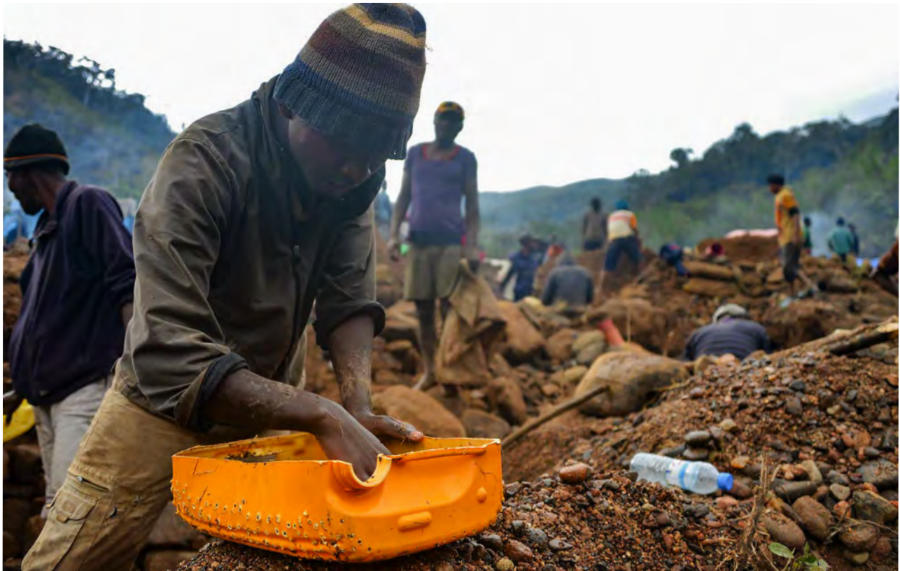
Figure 13. A young Malagasy miner searches for rubies in Zahamena with simple homemade tools: a pierced plastic oil can used as a sieve and an empty water bottle to store his gems. Photo by Vincent Pardieu/GIA.
