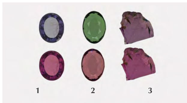
Figure 13. These photos show polished wafers under daylight-equivalent light (top) and incandescent light (bottom). Left to right: Samples Bl1 (1.487 mm thick), Gr1 (1.416 mm thick), and Pk1 (3.500 mm thick). Composite photo by Robison McMurtry.
