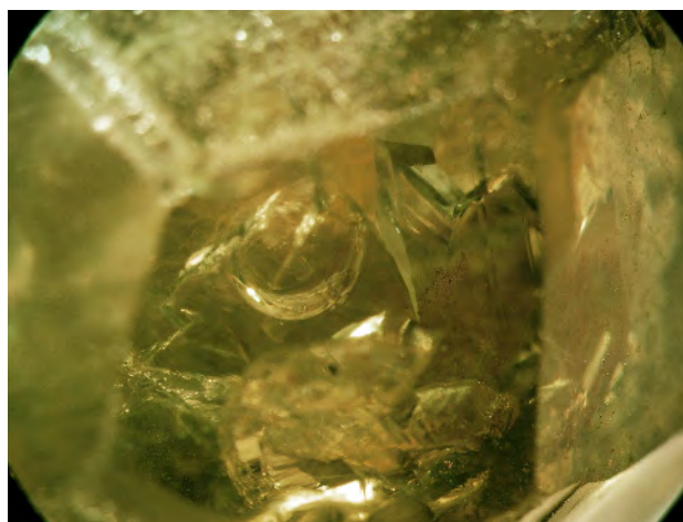
Figure 1. The demantoid crystal from Madagascar contains a giant two-phase fluid inclusion. The photomicrograph shows the FI cavity with its bubble trapped by the garnet. The bubble's diameter is around 2 mm. Photo by Michel Cathelineau.
