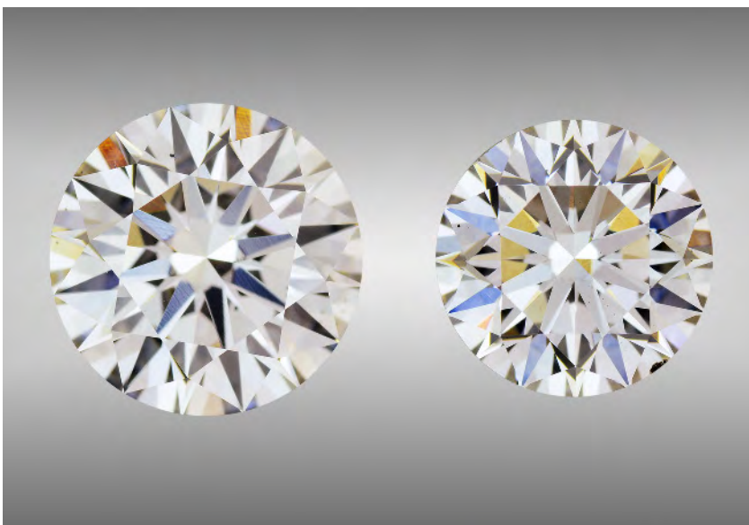
Figure 20. The I-color 3.23 ct round on the left (9.59–9.61 \times 5.83 mm) and H-color 2.51 ct round on the right (8.54–8.56 \times 5.43 mm) are the largest CVD synthetic diamonds GIA has tested.
