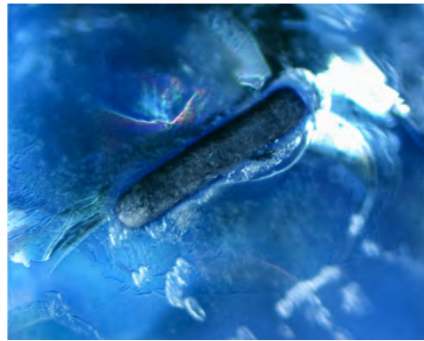
Figure 7. Prismatic and rounded rutile crystals, both orangy brown (left) and black (right), were encountered using a combination of dark-field and oblique illumination. Photomicrographs by Hanco Zwaan; field of view 0.7 mm (left) and 1.4 mm (right).
