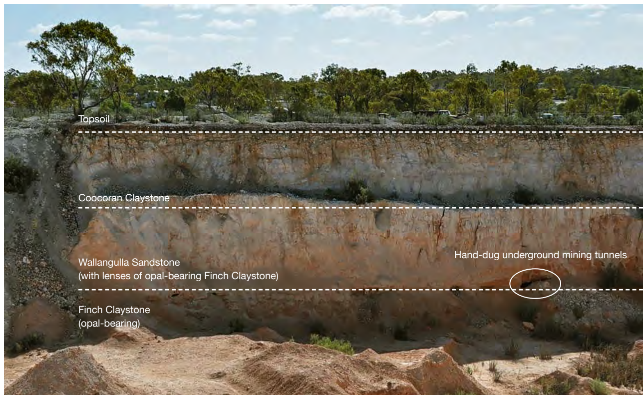
Figure 4. An exposed stratigraphic profile of the Lunatic Hill mine. Previous mining channels from the beginning of the 20th century can be seen at the boundary between the Wallangulla Sandstone and Finch Claystone units. The claystone is usually found at a depth of less than 30 meters. Photo by Vincent Pardieu/GIA.
