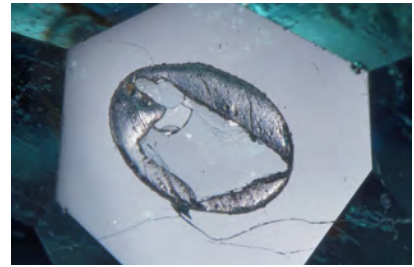
Figure 14. Examination of the drill hole in reflected light shows an emerald fragment intentionally placed in the opening, presumably to conceal the hole. Note the luster difference between the emerald and the resin filler. Field of view 3.57 mm.
