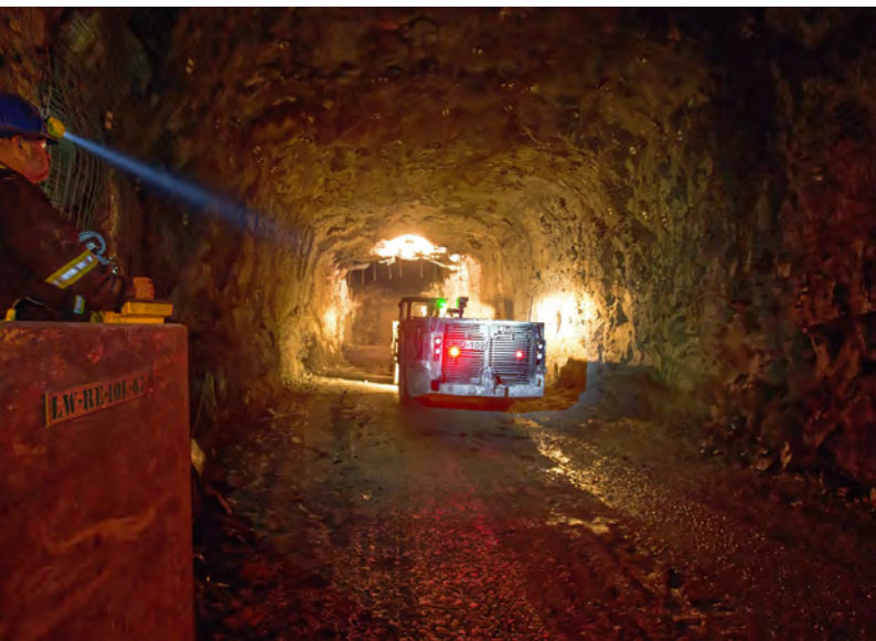
Figure 16. A long straight haulage tunnel is used to access the underground workings and haul kimberlite ore from the workings to the surface. Photo courtesy of Diavik Diamond Mine.
