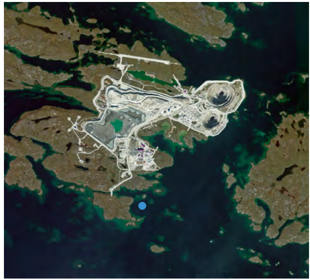
Figure 6. This photo, taken from space in August 2014, shows the A154 (top) and A418 (bottom) open pits on the right side of the image. Since the kimberlite pipes were initially covered by Lac de Gras, it was necessary to first construct dikes around the pipes to prevent water from flooding the open pits and underground mine workings. The A21 kimberlite pipe is also under the lake—its location is indicated by the blue dot. Photo courtesy of Diavik Diamond Mine.
