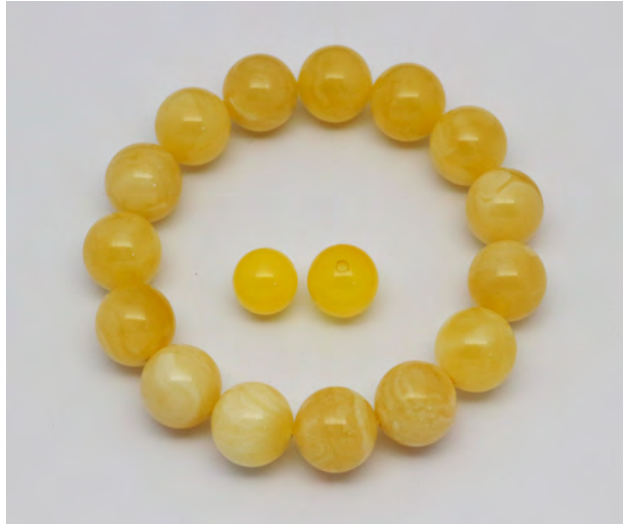
Figure 19. The two bright yellow beads in the center, 8 mm and 9 mm in diameter, were treated by steam dyeing, while the bracelet contains natural-color amber. Photo by Jiewan Huang.
