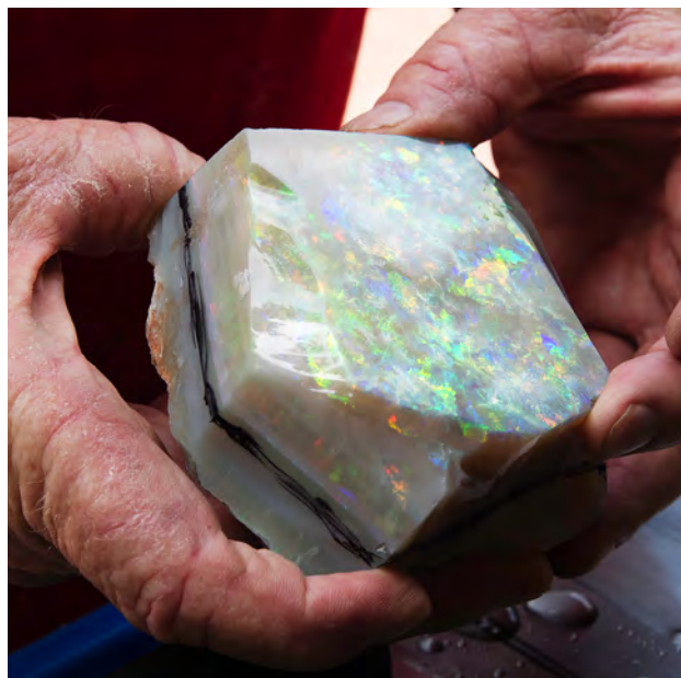
Figure 4. The gem rough has been scribed with a black marker and is ready for the cut. Photo by Eric Gofreed/Eric Gofreed Photography.
