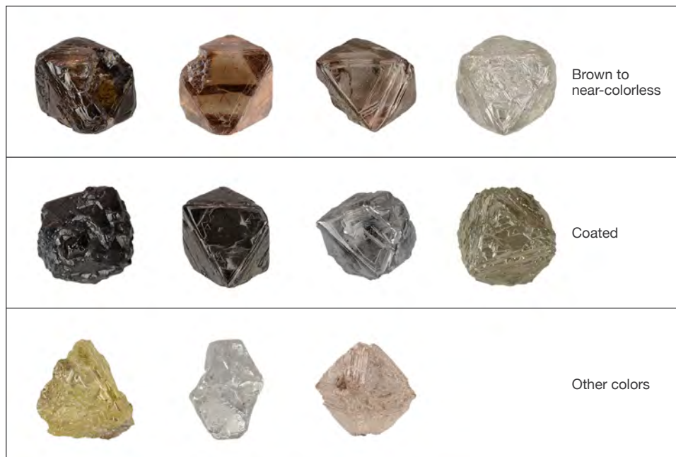
Figure 24. Representative colors of Diavik rough diamonds, ranging from colorless to brown to yellow with one pink crystal. Also shown are several coated crystals. Photos by Jian Xin (Jae) Liao.
