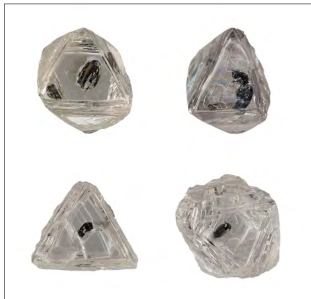
Figure 25. Several of the Diavik diamonds exhibited dark inclusions, presumably sulfide minerals. Photos by Jian Xin (Jae) Liao.
