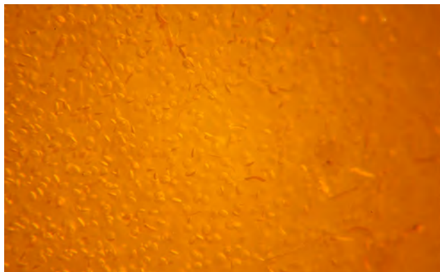
Figure 21. Left: The squashed bubbles are induced by steam treatment, and the red filaments are possible traces of residual dye. Photomicrograph by Fen Liu; field of view 2.95 mm. Right: The dark orange color zone among the bubbles, unrelated to the cracks, indicates that the color zone was introduced by dyeing. Photomicrograph by Shufang Nie; field of view 2.95 mm.
