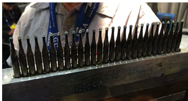
Figure 35. This cassette, which can hold up to 56 melee at one time, is shown holding 28 larger stones. Photo by Tao Hsu.
