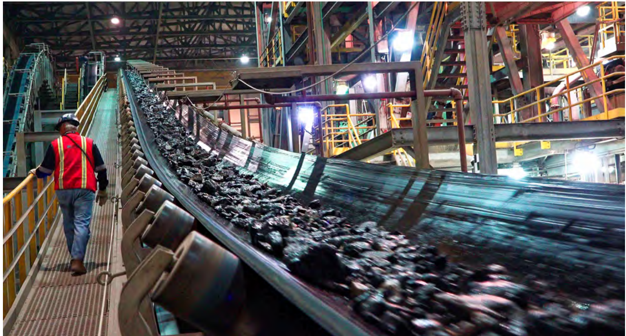
Figure 21. The kimberlite ore is transported by conveyor belts between different stages of the processing sequence. Photo by James Shigley.
