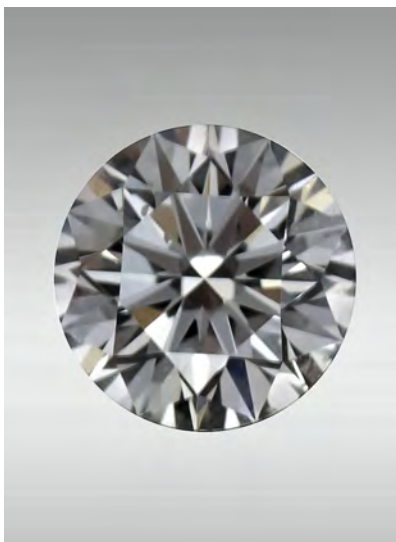
Figure 3. This 0.40 ct, D-color type IIa round brilliant diamond showed very bright red fluorescence due to strong emission peaks from the nitrogen-vacancy centers.
