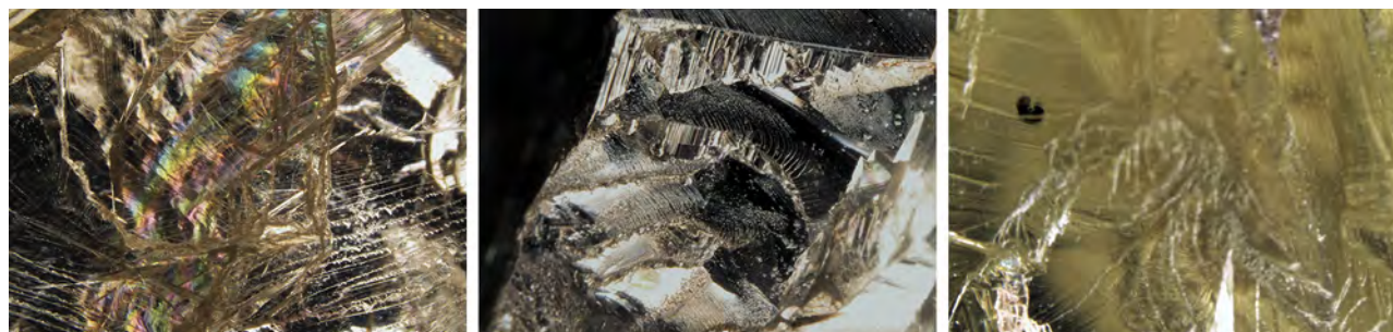
Figure 2. Iridescent color can be seen along the cleavage plane on one side of the stone (left). Dissolution pits are observed on the surface of the yellow rough (center), and a dark mineral inclusion is clearly visible near the surface (right). Field of view 14.52 mm (left), 4.79 mm (center), and 7.19 mm (right).
