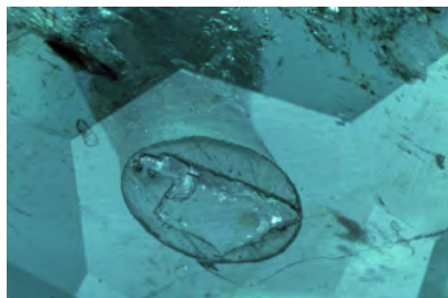
Figure 12. With microscopic examination, the circular outline of the drill hole is apparent on the pavilion facet of the emerald. Field of view 4.08 mm.
