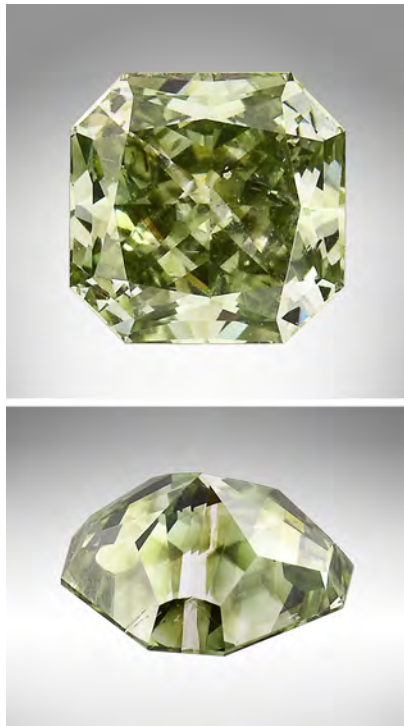
Figure 18. This 0.42 ct green HPHT synthetic diamond displayed strong growth sectors that were observed without magnification.
