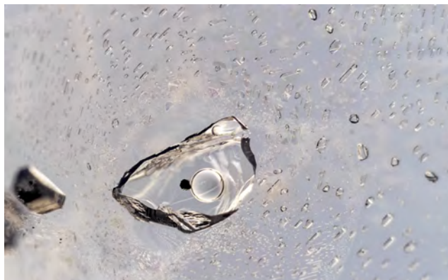
Figure 14. Left: A large fluid inclusion containing a CO 2 gas bubble and a marcasite crystal. The primary inclusion is surrounded by smaller inclusions that make up a healed fissure. Right: When the sample was gently heated, the gas bubble disappeared as the gas and liquid homogenized. The sample is illuminated using diffused backlighting. Photomicrographs by Victoria Raynaud; field of view 1.20 mm.
