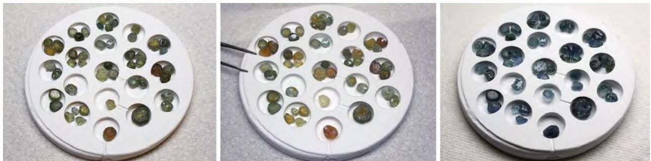
Figure 20. Rough sapphires from Rock Creek before and after two rounds of heating. Left: The material before heating. Center: The same sapphires after the oxidizing "fancy burn." Right: The same sapphires after the reducing "blue burn." Photos courtesy of Gem Mountain Sapphire Mine.
