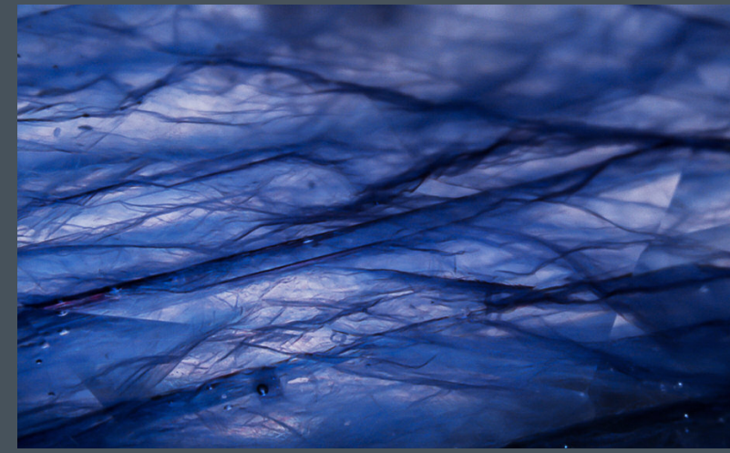
Cobalt-doped lead glass is used to bind colorless corundum in this manufactured product. Blue color concentrations from the cobalt glass and gas bubbles are visible in the microscope. Field of view 7.84 mm.
