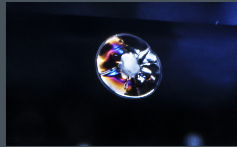
A whitish altered mineral crystal and discoid tension crack with a healed fringe are proof of heat treatment in this metamorphic blue sapphire. Field of view 2.12 mm.
