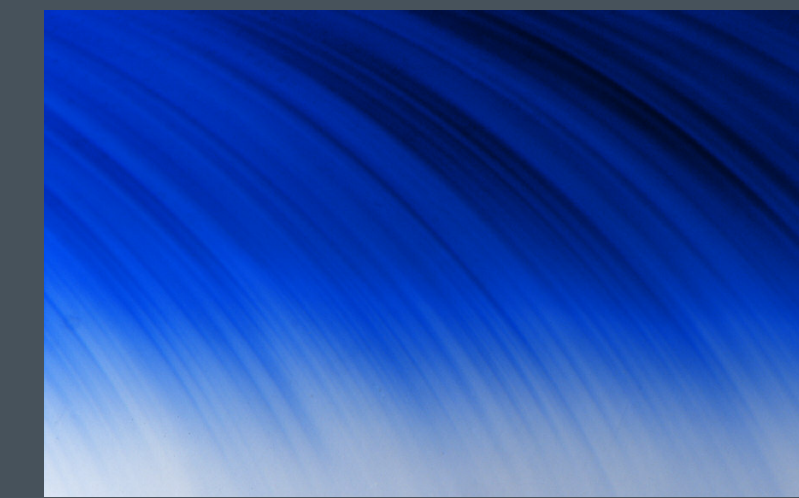
Curved color banding is diagnostic for flame-fusion material, as in this blue synthetic sapphire. Field of view 4.11 mm.
