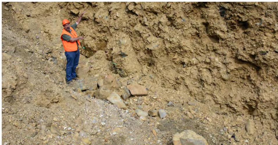
Figure 13. Dr. Keith Barron, geologist and owner of Potentate Mining, shows the sapphire- and gold-bearing mudflow at Eureka Gulch. Compared to the well-sorted alluvial gravel layer at Eldorado Bar, the ore zones contain much finer-grained soils along with coarser gravel and boulders. Photo by Andrew Lucas.
