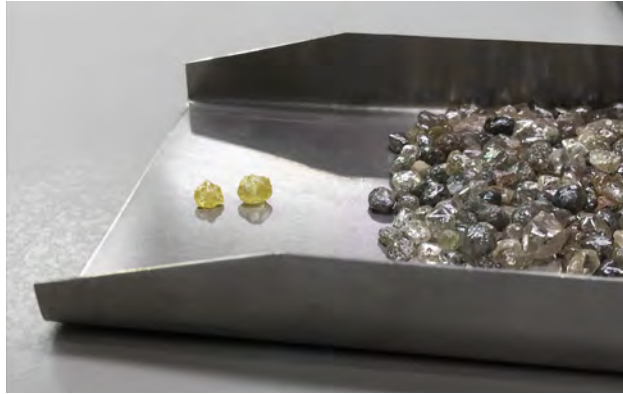
Figure 8. Two yellow cubo-octahedral diamonds separated during recovery sorting in the processing plant at the Lomonosov mine. Photo by Karen Smit.
