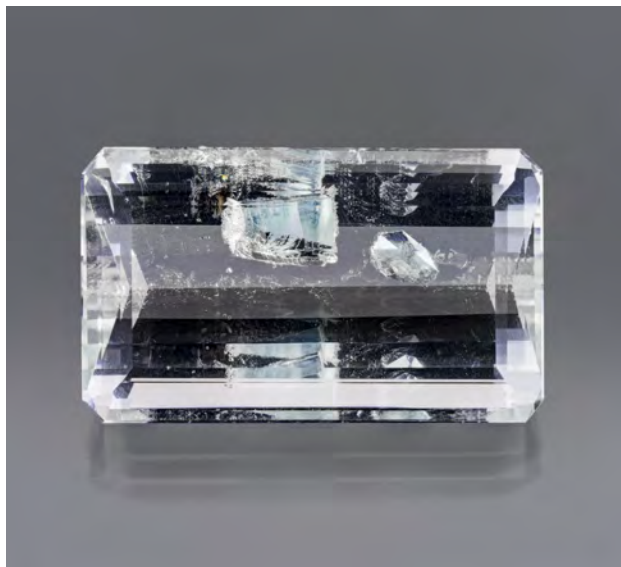
Figure 3. This 57.56 ct rock crystal quartz hosts two large euhedral chlorapatite crystals. Photo by Kevin Schumacher.
