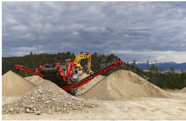
Figure 14. Dry screening/concentrating plant near Sapphire Gulch. Here, sapphires are mined on the hill slopes and benches rather than the stream beds. Currently, Potentate recovers sapphires from the concentrated +1/8 in. to -1 in. material. They are stockpiling the -1/8 in. undersized material. Photo by Andrew Lucas.
