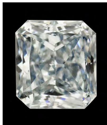
Figure 21. This 0.33 ct Fancy blue diamond was confirmed to be a composite of CVD synthetic type IIb diamond overgrowth on a natural type Ia substrate.
