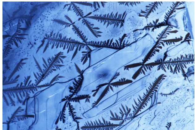
Figure 9. Fiber-optic illumination reveals dendritic inclusions of a manganese oxide-hydroxide compound trapped within a fracture. Photomicrograph by Charuwan Khawpong; field of view 1.05 mm.
