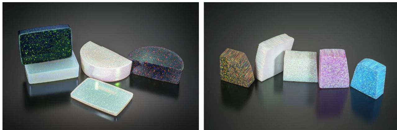
Figure 11. This new plastic opal imitation (left) shows a very pleasing play-of-color that does not have the classic “snakeskin” columnar structure one would expect to see in traditional polymer-impregnated synthetic opal produced by Kyocera (right). The largest sample of plastic imitation opal in the left photo weighs 227 grams, and the largest sample of synthetic opal in the right photo weighs 65 grams. The rectangular black block in the photo on the left is 9.7 cm in length.
