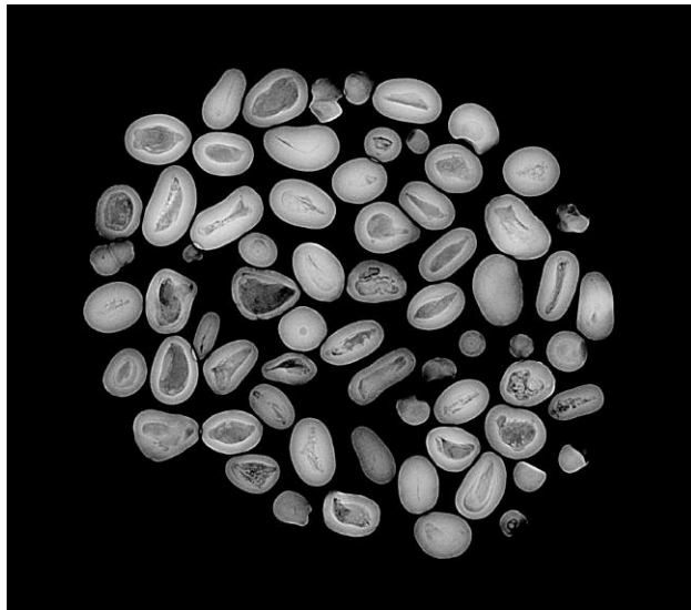
Figure 52. RTX analysis of tiny loose akoya NBC pearls revealed void-like structures in most of them. Image by Promlikit Kessrapong.
