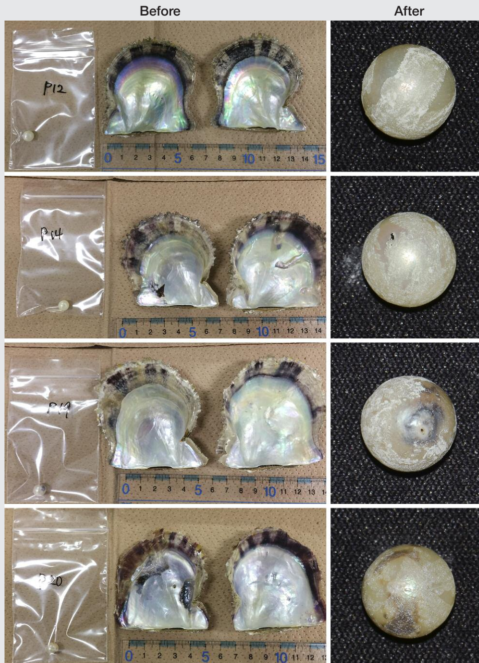
Figure B-1. The akoya pearl samples used in this study. The photos on the left show the specimens in plastic bags (along with the host oysters) before the powder samples were obtained. Photos by K. Saruwatari. The photos on the right, taken after the powder samples were obtained, show severely damaged pearls and exposed inner nuclei. Photos by S. Nagai.
