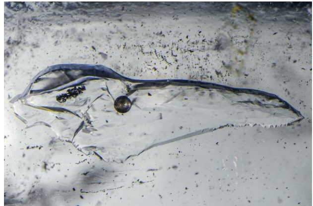
Figure 16. The metallic-looking bubble has floated toward the left end of the fluid inclusion chamber. Photomicrograph by Nathan Renfro; field of view 7.42 mm.
