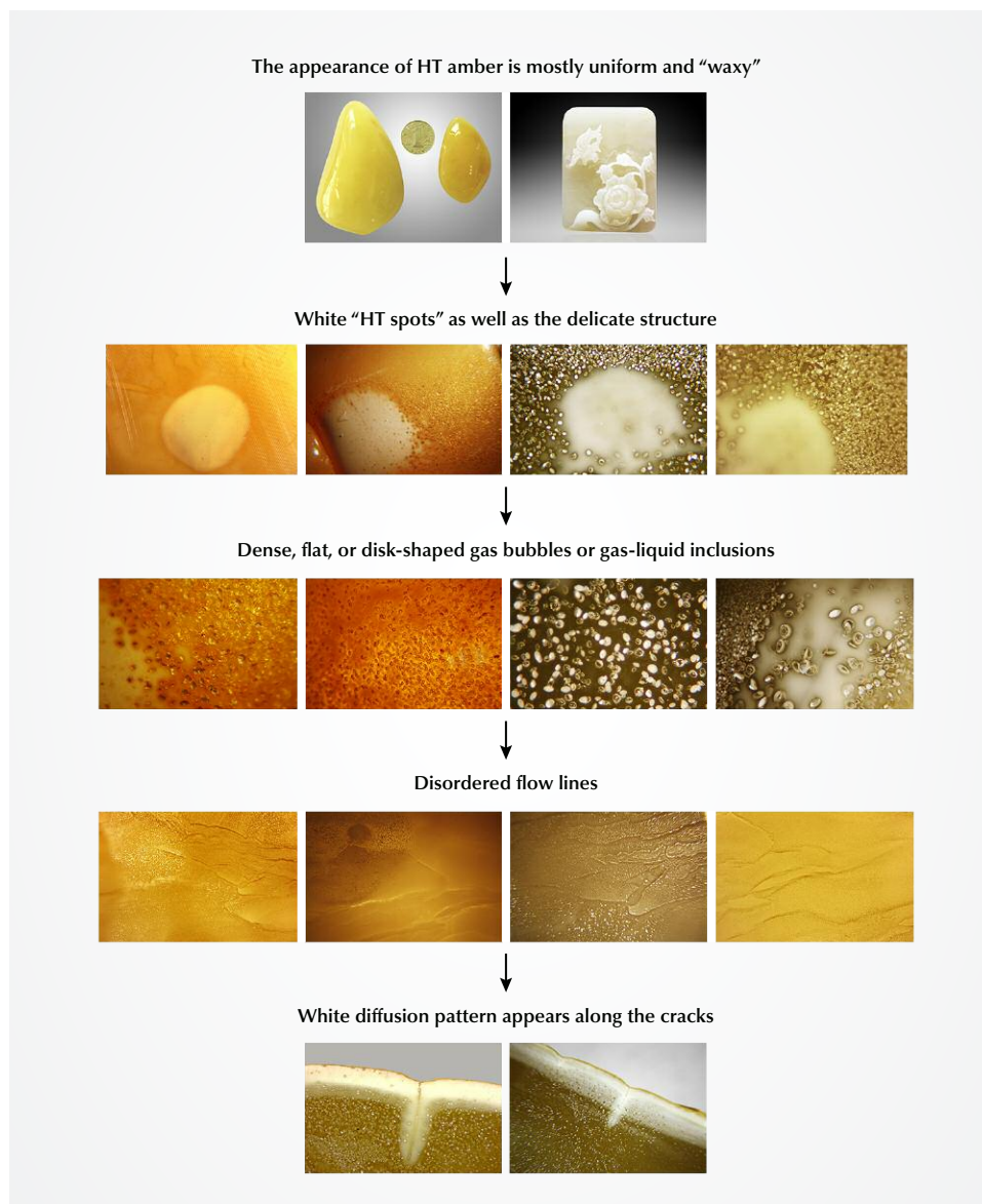
Figure 17. Flowchart for the identification of hydrothermally treated amber. Photos by Yamei Wang.
