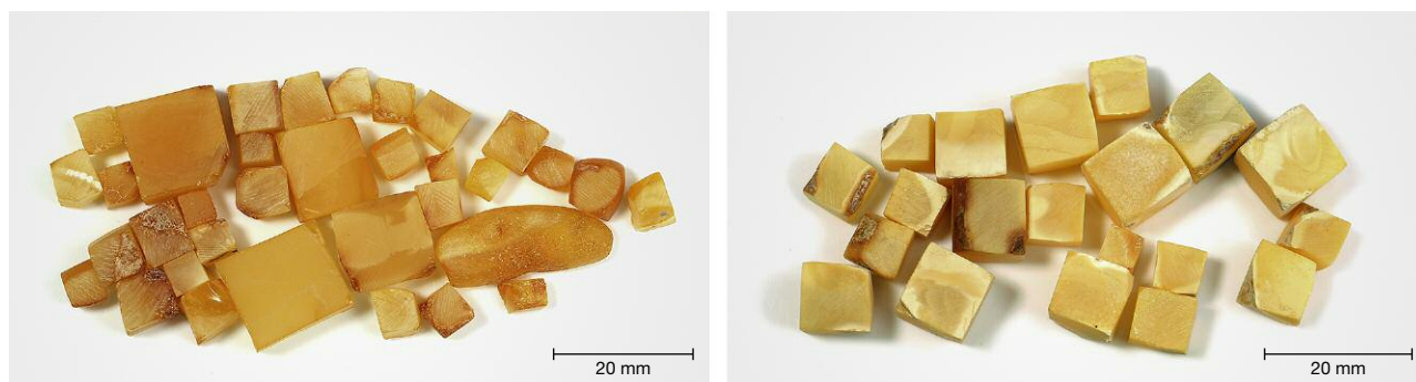
Figure 15. Semi-finished amber before and after hydrothermal treatment, photographed at the factory. Photos by Yamei Wang.
