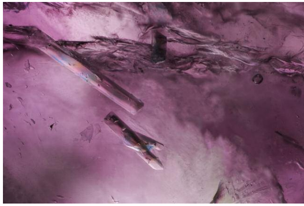
Figure 11. The longest inclusion in this photomicrograph of a Russian alexandrite was conclusively identified as tourmaline. This tourmaline inclusion exhibits a well-formed prismatic/rod-like crystal shape. Darkfield illumination. Photomicrograph by Jonathan Muyal; field of view 1.44 mm.
