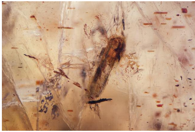
Figure 5. This colorful inclusion scene showcases an anthophyllite crystal inclusion, which exhibits high transparency, several cleavage planes, and a thin/bladed prismatic crystal form. Photomicrograph by Jonathan Moyal; field of view 2.34 mm.
