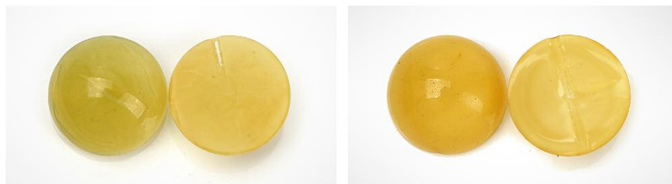
Figure 16. Left: HT amber beads. Right: The roasted HT amber with enhanced color. Samples were collected from the factory. Photos by Yamei Wang.
