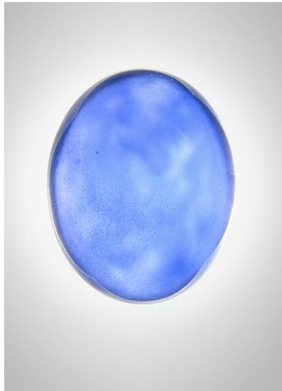
Figure 19. Mottled blue patterns were observed in the synthetic sapphire against transmitted illumination through a diffuser plate.
