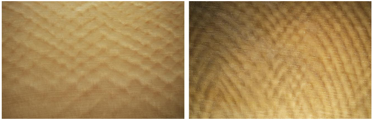
Figure 10. Left: Elephant ivory with Schreger lines intersecting at an average angle of 109°; field of view 19.27 mm. GIA Collection no. 4287. Right: Mammoth ivory with Schreger lines intersecting at an average angle of 69°; field of view 19.27 mm. Part of GIA Collection no. 19267, donated in 1995 by Richard Marcus of Mammoth Enterprises, Inc.
