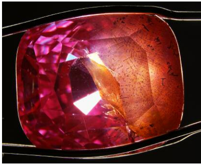
Figure 20. This 14.36 ct pink-orange synthetic sapphire contains large fractures with orange staining and some partially crystallized foreign material. Field of view 15.26 mm.
