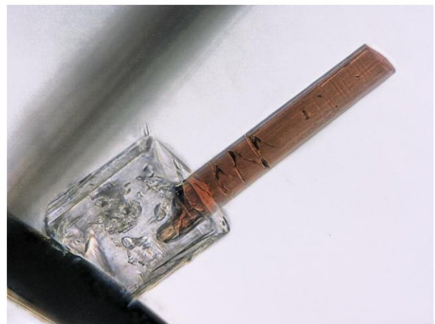
Figure 12. A phenakite specimen from Ambohimambola, Madagascar, contained a tourmaline with a spiral growth feature and a colorless crystal. Photomicrograph by Kimberly Abruzzo; field of view 0.88 mm.
