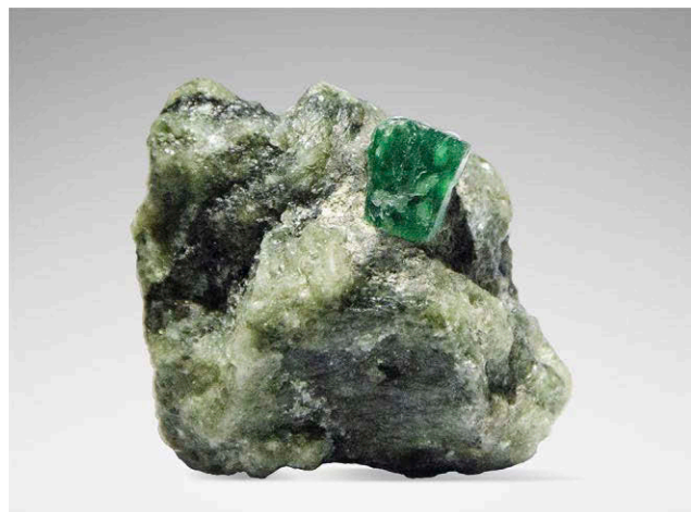
Figure 4. An emerald crystal specimen in matrix from the Mingora mine in Swat Valley. The emerald crystal measures about 7 \times 7 \times 8 mm (left). The matrix (right) mainly consists of dolomite (light green), magnesite + talc (white), graphite + talc (grayish black), and pyrite (pale brass-yellow), identified by Raman analysis. Photos by Hongshu Guo (left) and Xiaoyan Yu (right).
