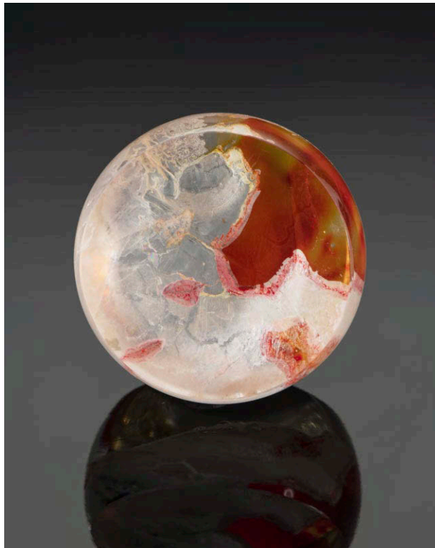
Figure 6. This 226 ct round tablet of quartz contains an orange and yellow resin-filled fracture that convincingly imitates natural iron oxide mineral staining in quartz. Photo by Robert Weldon; courtesy of Mike Bowers.
