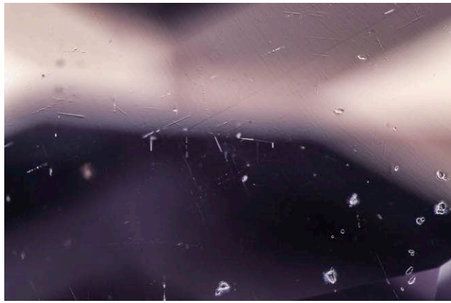
Figure 18. Left: When the pinkish purple sapphire was viewed under darkfield illumination, the only inclusions visible underneath the table were zircon crystals and rutile needles. Right: Examining the same area with fiber-optic light revealed unknown dendritic inclusions. Photomicrographs by Ezgi Kiyak; field of view 2.90 mm.
