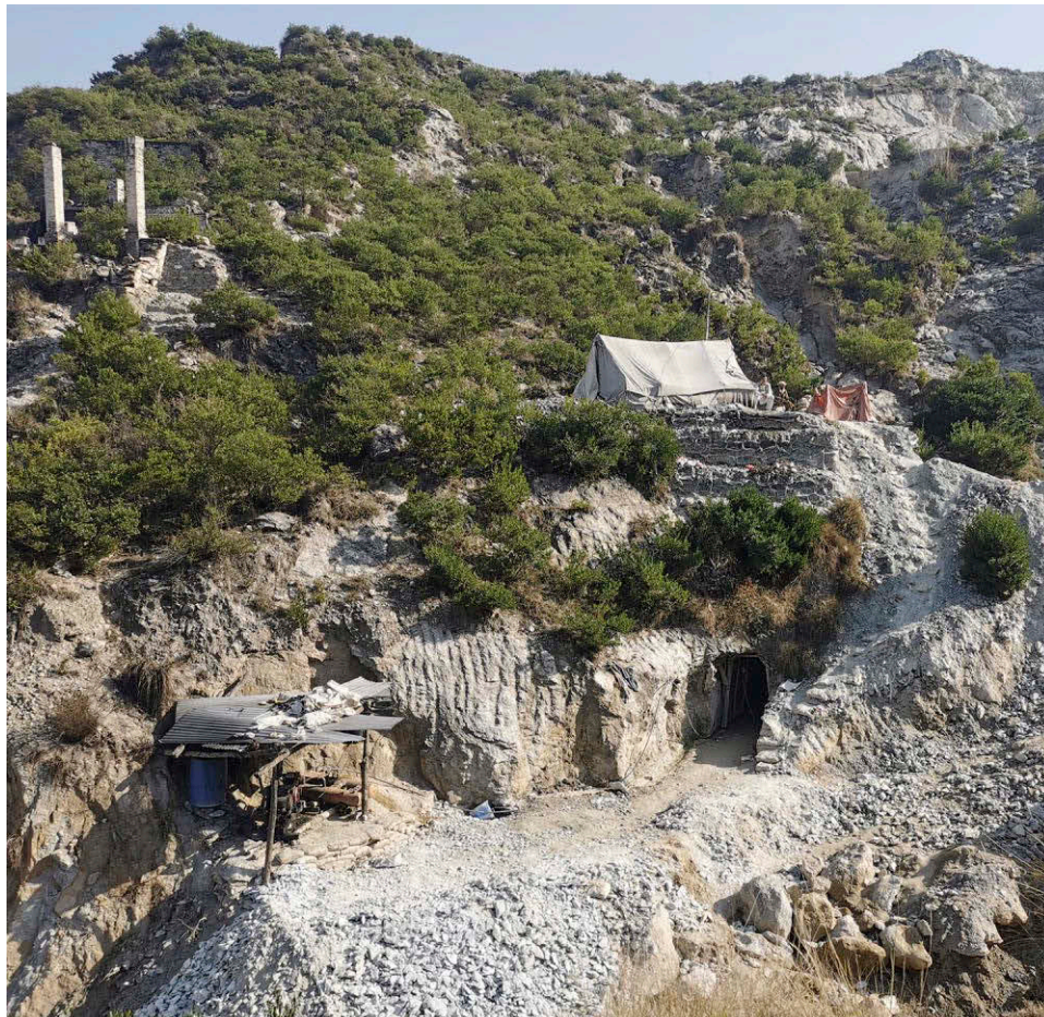
Figure 5. Top: The Mingora mine now has 30 active tunnels. Bottom left: The tunnels are dug in horizontal and slightly downward directions. Bottom right: The miners collect emeralds with hydraulic jackhammers and handpicks. Photos courtesy of Cloud Walker Jewel, Inc.
