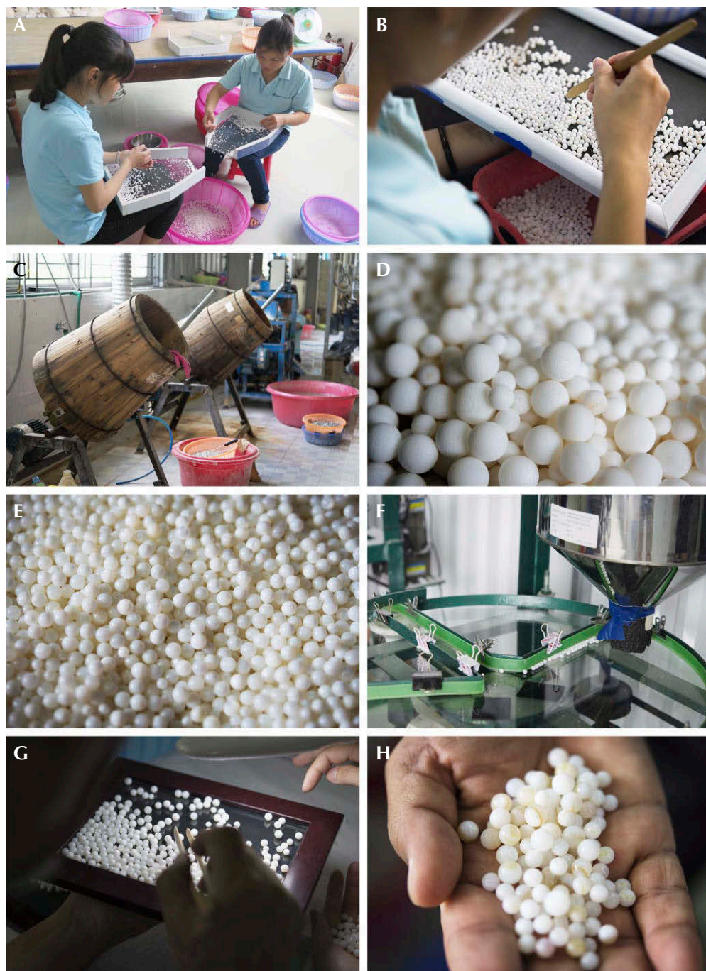
Figure 4. Photos from inside the factory show the stages of nuclei processing. Quality checks by the staff to remove any nuclei that need further processing (A and B), wooden tumblers for removing the powder from the surface and imparting a final finish (C), matte-surfaced nuclei prior to insertion into the drums (D), significantly improved surface luster after drum processing (E), the machine that checks the roundness of the fully processed nuclei (F), the final color grading/sorting step (G), and a selection of washboard mussel nuclei showing clear yellow banding (H). Photos by Nuttapol Kitdee (A, C, E), Nick Sturman (B, D), and Kwanreun Lawanwong (F).
