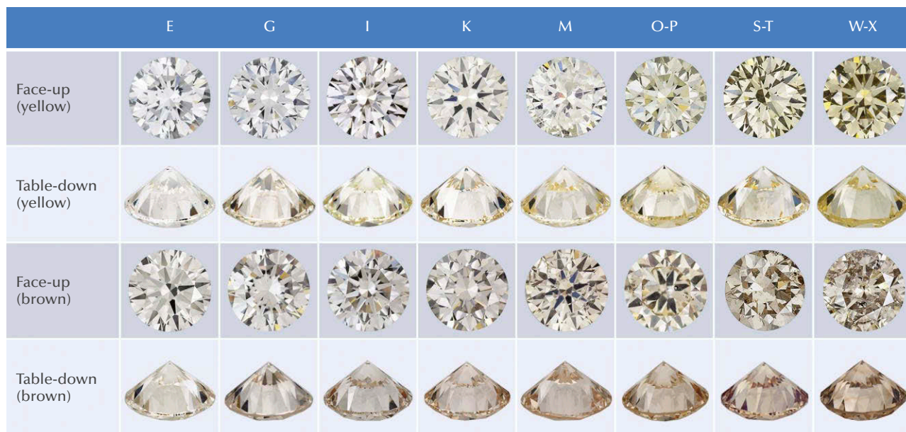
Figure 2. The color grades of D-to-Z diamonds are generally assessed in the table-down position (King et al., 2008) but admired in jewelry in face-up orientation. While most D-to-Z diamonds show a yellow coloration, a small percentage (about 5% overall) show a brown color.
