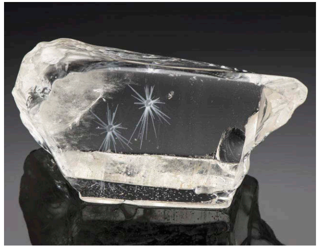
Figure 10. This 724 ct rock crystal quartz contains two manufactured inclusions induced by a 3D subsurface laser-engraving process. Photo by Robert Weldon; courtesy of Mike Bowers.
