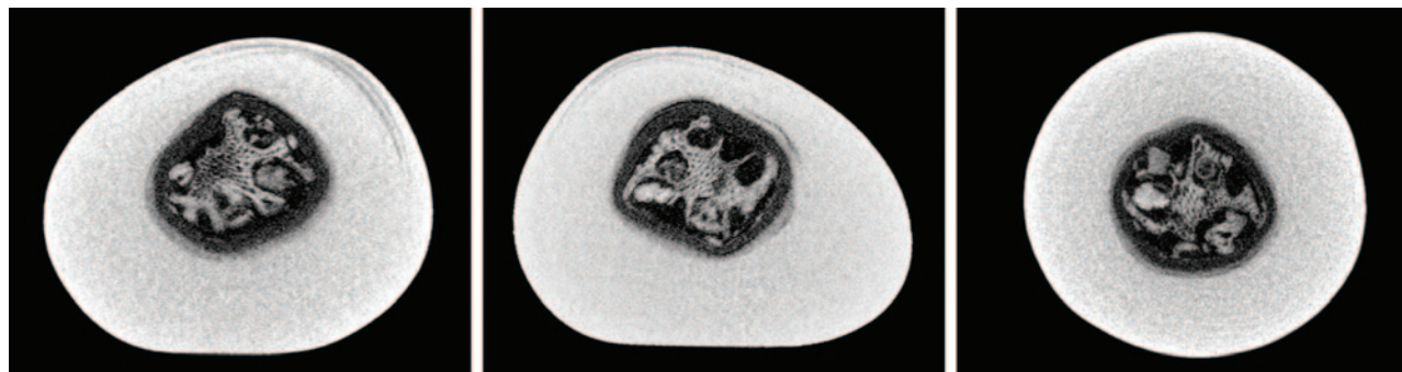
Figure 12. \mu -CT slices in three directions of sample 6-4 revealed a porous-looking structure in the main feature, possibly resembling the structure of coral from the Melithaea genus, a fan coral distributed throughout the tropical Indo-Pacific region.
