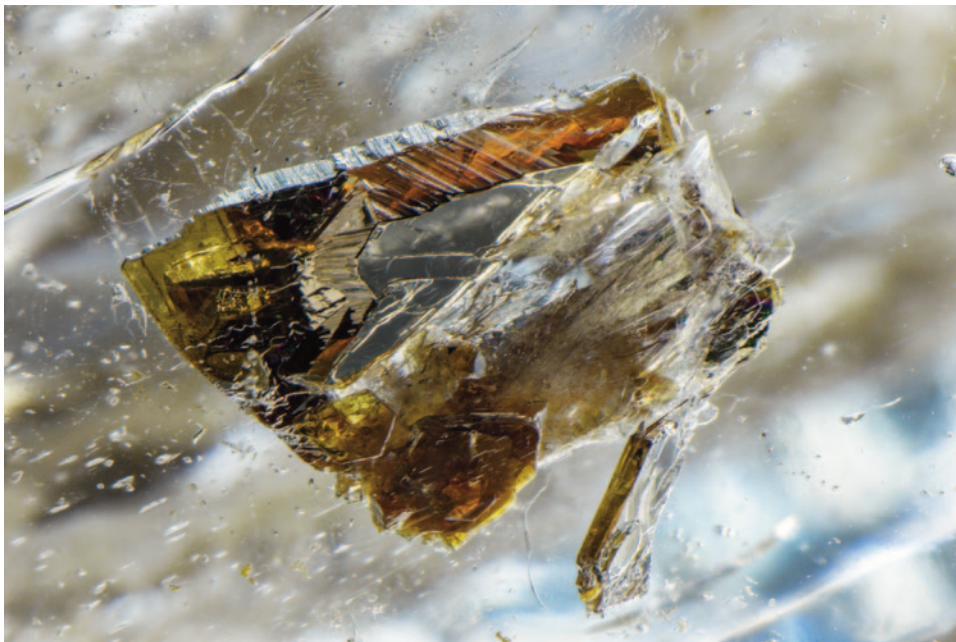
Figure 13. This prominent 6 mm crystal of phlogopite mica is hosted by the Pakistani topaz. Photomicrograph by Nathan Renfro; field of view 9.09 mm.
