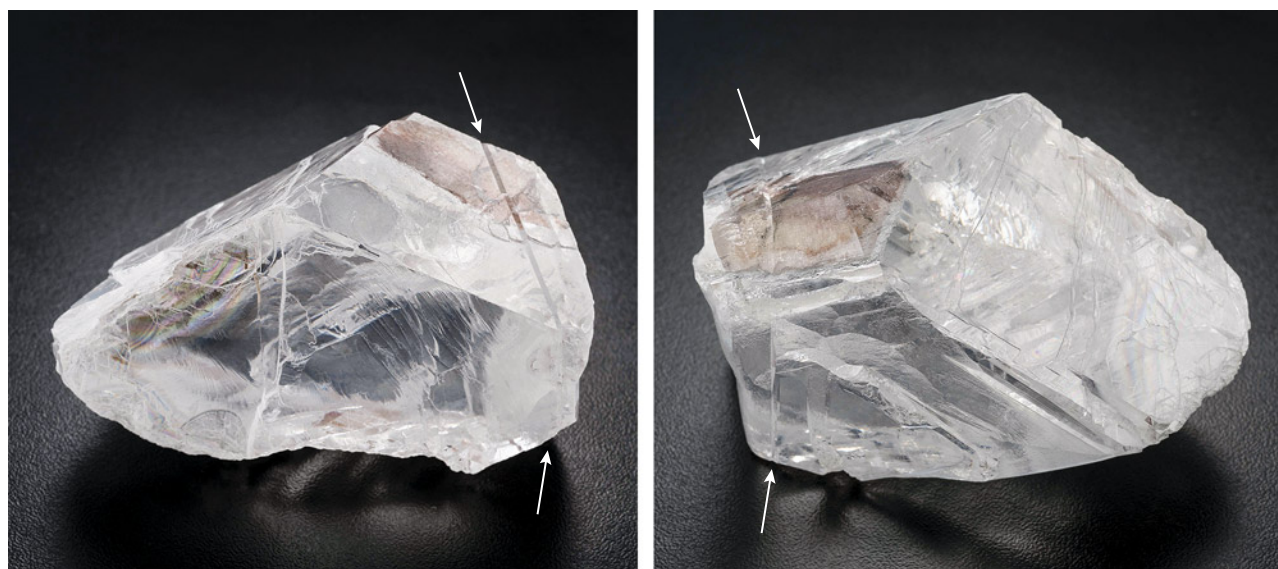
Figure 4. Two views of a large rough diamond with a pronounced mechanical twin plane. This 812 ct diamond, named the Constellation, has both freshly cleaved surfaces (left) and natural resorbed surfaces (right). Both views show a kink that wraps around the entire surface and defines an internal {111} twin plane where the crystal orientation is reversed with respect to the rest of the diamond. The diamond is 6.6 cm in its longest dimension. Photos by Jian Xin (Jae) Liao.
