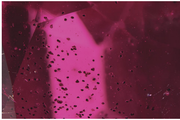
Figure 13. Numerous natural-looking dark red solid inclusions were observed in a flame-fusion laboratory-grown ruby. Photomicrograph by Ezgi Kiyak; field of view 2.9 mm.
