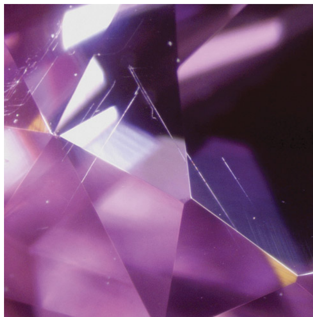
Figure 95. Unaltered tubes in the heated purplish pink sapphire. Photomicrograph by Ugo Hennebois; field of view 2 mm.
