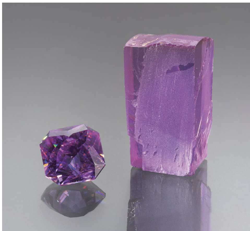
Figure 89. Faceted and rough synthetic wakefieldite in LED lighting with 6400K color temperature. The faceted stone is 5.04 ct. Photo by Adriana Gudino; courtesy of Arya Akhavan.
