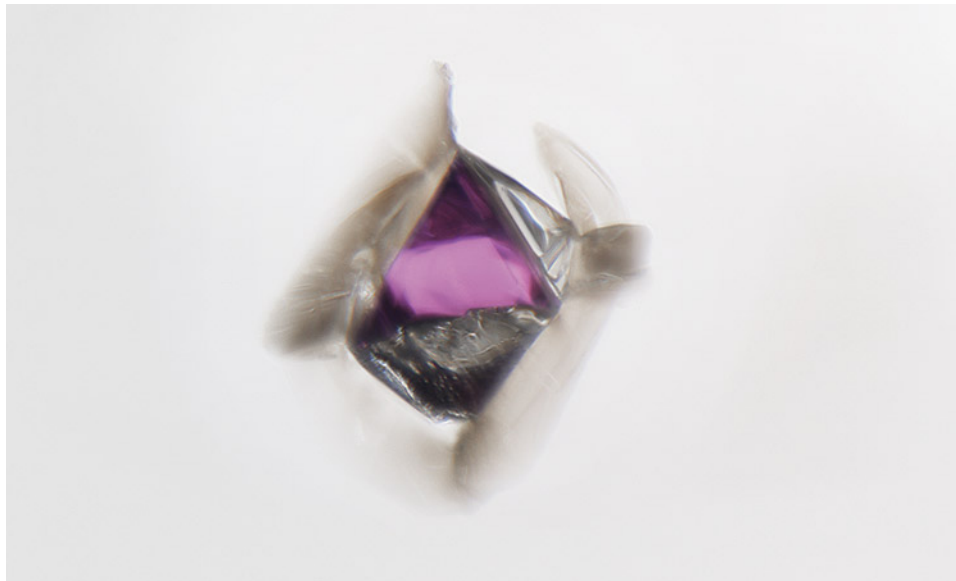
Figure 11. A purplish pink xenomorphic octahedral garnet crystal seen in a diamond. Note the trigons on the upper right octahedral face and stress fractures around the intersections of the crystal faces. Photomicrograph by Britni LeCroy; field of view 1.26 mm.
