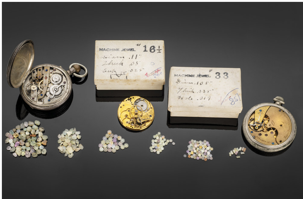
Figure 6. Watch bearings fashioned out of Montana sapphires in various stages of completion. The leftmost pile contains rough sapphires ready for fabrication, and the pile second from the left contains sapphires ground to wafers of standard thickness to be drilled out to produce bearings. The four piles to the right show finished natural sapphire watch bearings. Photo by Robert Weldon; courtesy of the Sapphire Gallery.
