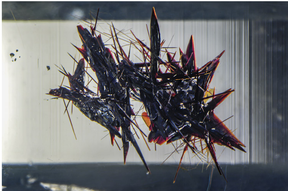
Figure 16. None of the analytical techniques at our disposal were able to conclusively identify the mineral making up the 7.20 mm inclusion cluster. The distinctive morphology shown by these inclusions strongly suggests that the cluster is composed of columbite-(Mn) crystals. Photomicrograph by Nathan Renfro; field of view 10.28 mm.
