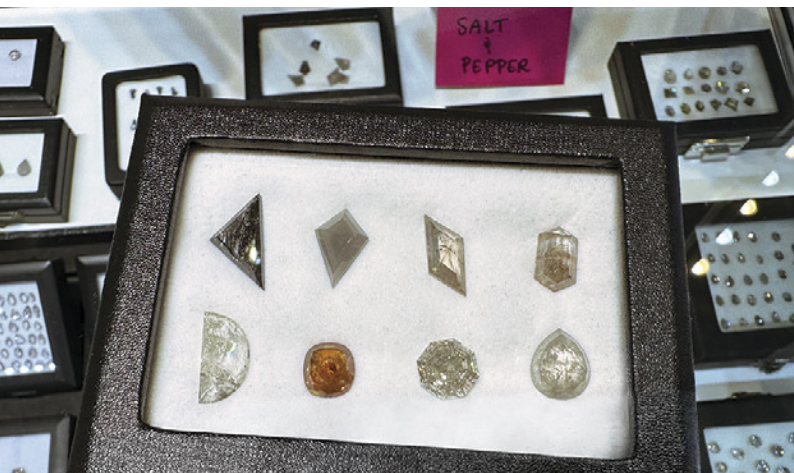
Figure 5. “Salt and pepper” diamonds containing eye-visible inclusions. Photo by Jennifer Stone-Sundberg; courtesy of Misfit Diamonds.
