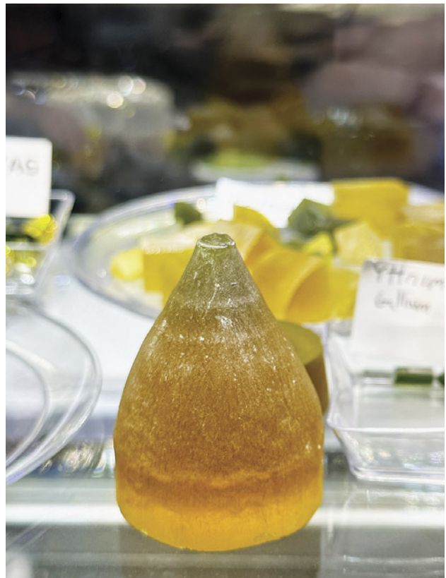
Figure 53. The top of a YAG boule doped with cerium and neodymium and produced by the Czochralski method, measuring approximately 36 mm in diameter and 45 mm tall. Parts of the boule that cannot be used for scientific purposes can be sold to the gem and jewelry trade for faceting. Photo by Lisa Kennedy; courtesy of Turtle’s Hoard.
