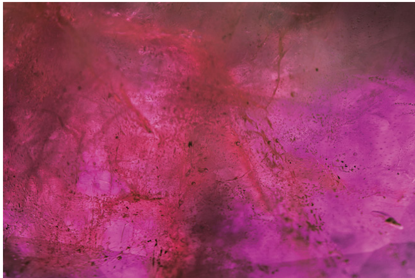
Figure 27. Fingerprints resulting from flux-assisted heating of a beryllium-rich flux. Field of view 7.19 mm.
