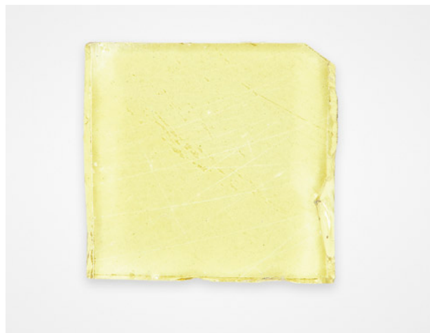
Figure 29. Sample 1162, a \text{Ni}^{3+} -doped sapphire cut from boule SS9. The c -axis is in the plane of the wafer, which measures 10.0 \times 10.0 \times 2.14 mm. Photo by John L. Emmett.
