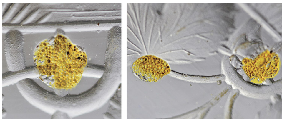
Figure 21. Residues of the yellow fixation layer on the glass substrate of the beaker in Passau showing an uneven surface with a bubble-like texture; the yellow residual materials measure about 3 mm in diameter. Photos by H.A. Gilg.
