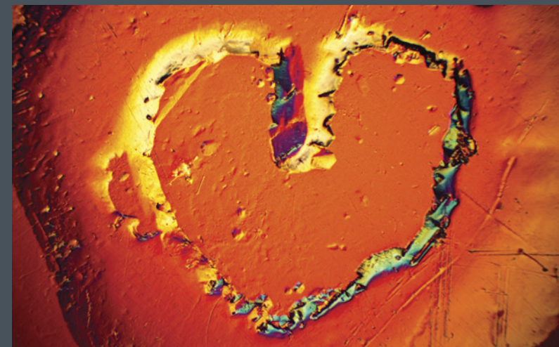
This morganite crystal shows a heart-shaped etch feature on the pinacoid face, as seen using differential interference contrast microscopy. Field of view 1.5 mm.
