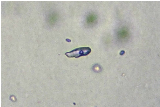
Figure 14. The white cross inclusion in the rock crystal contained this two-phase inclusion, in which the bubble had a diameter of approximately 2 \mu\text{m} and exhibited Brownian motion. Photo by Shu-Hong Lin; field of view 65 \mu\text{m} .
