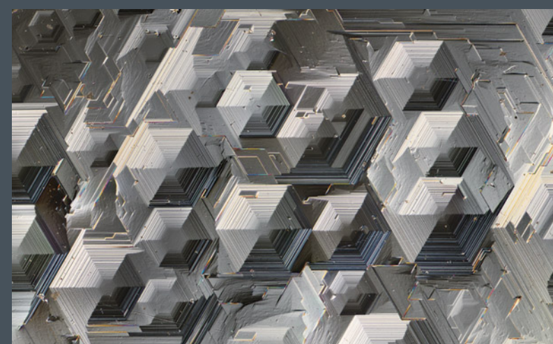
Growth hillocks reveal the hexagonal crystal structure on the pinacoid face of this aquamarine from Pakistan using differential interference contrast microscopy. Field of view 2.32 mm.
