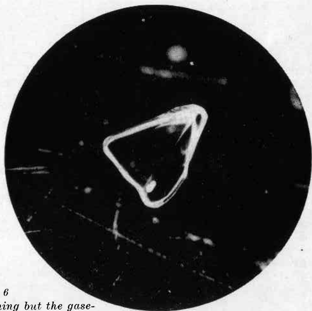
Fig. 5 Irregular liquid inclusion in an amethyst at normal room tempera- ture. 300x.
