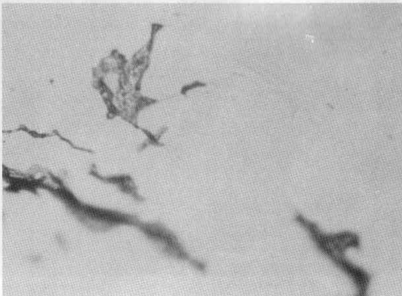
Figure 7a. This picture photographed in bright field lets the microscopist only vaguely guess some faint structural peculiarities in a yellow fluorspar from Switzerland. Photo ocular pol. 10x. Achromatic objective pol. 6.3/0.16 Huygens. Magnification 63x.
