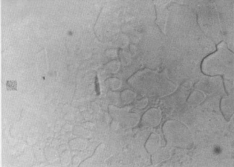
Figure 8a. Partly healed flat fissure in a yellow beryl from Madagascar photographed in bright field shows inhomogeneities very faintly, making it almost impossible to understand their nature. Photo ocular pol. 10x. Achromatic objective pol. 25/0.45 Huygens. Magnification 250x.
