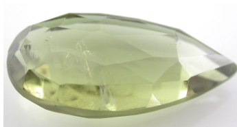
Figure 16.32.1: Color-changing diaspore from green in daylight to brown in incandescent light - also known as “Zultanite” in the gem market.
