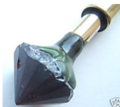
Figure 17.2.3: The pavilion break facets. Notice a large pit. This pit has to be removed by grinding all the facets a bit more.
