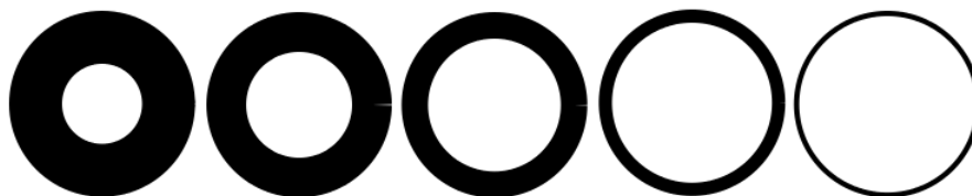
Figure 11.7.4: From left to right: casted rims (shadows) by a brilliant cut gemstone for decreasing RI difference between liquid and gemstone. From thick to fine
