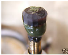
Figure 17.2.7: Beginning of cutting the break facets. Notice that the break facets don't align perfectly with the girdle. This is not uncommon. There is an index micro-adjuster called a cheater on the machine. Use the cheater to correct the alignment.
