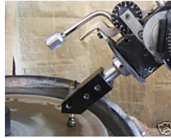
Figure 17.2.10: The dop is positioned perpendicular to the lap with the table block.
