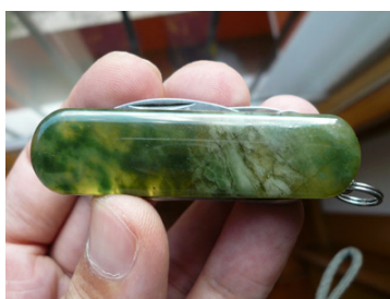
Figure 16.70.2.3: Californite used as a material for knife scales. The part lighter in color and more opaque (right side) is enriched in chlorite.
