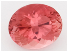
Figure 16.14.11: Ramped up to 520° C over a three hour period. Held at 520° C for two hours, followed by cooling (same stone)
