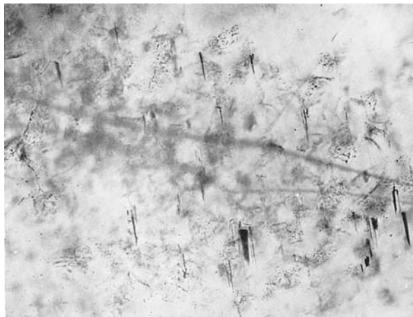
Figure 24.22 Feathers and needles in a Linde synthetic emerald
