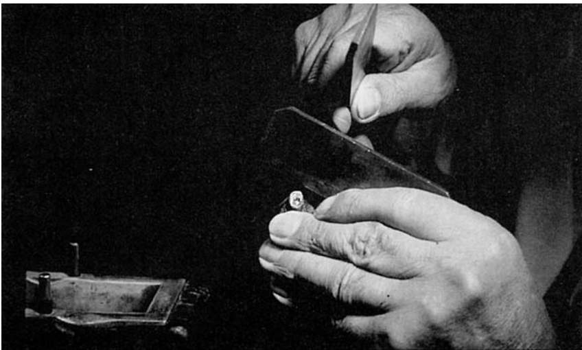
Figure 30.29 The cleaving blade in position ready for the blow which will cause the diamond to split in two (courtesy of De Beers)
