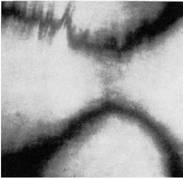
Figure 24.5 Anomalous double refraction (tabby extinction) in a synthetic spinel
