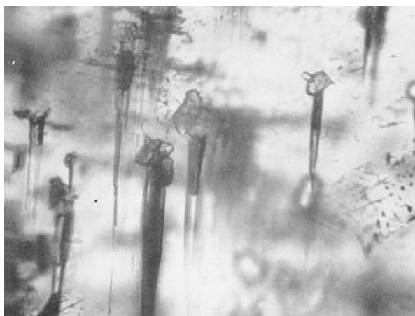
Figure 24.23 Conical cavities capped with phenakite crystals in a Linde synthetic emerald
