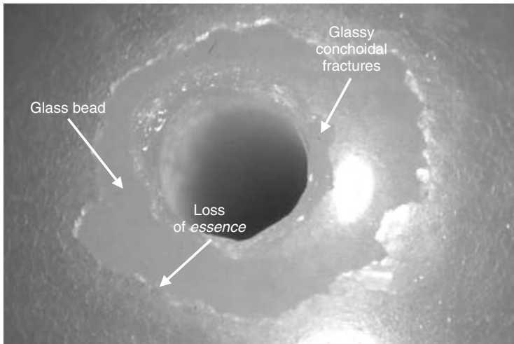
Figure 28.17 Identifying appearance of the stringing channel in essence coated solid glass bead imitation pearl
