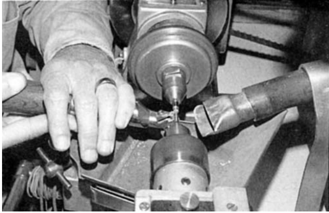
Figure 30.33 The bruter rondisting a sawn octahedral diamond. A corner of the other section of the sawn stone is clamped in a dop stick and used as the cutting tool (courtesy of Monnikendam).
