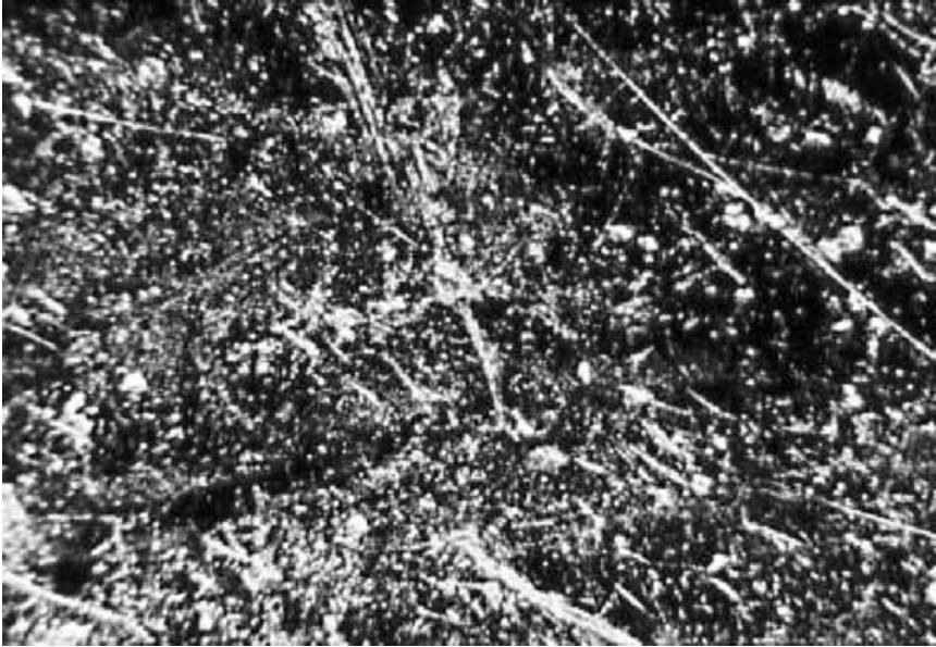
Figure 31.1 Scratched 'bubble' included, iridescent surface patch of magnesium fluoride located under the girdle of a coated diamond ( \times 40 , tangential illumination)
