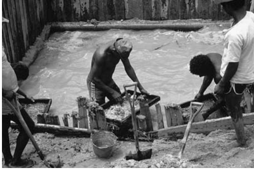
Figure 1.29 Washing gravel and hand-picking gems from the alluvial deposits at Marambaia, Minas Gerais, Brazil. The valley is well known as a source of fine aquamarine and chrysoberyl
