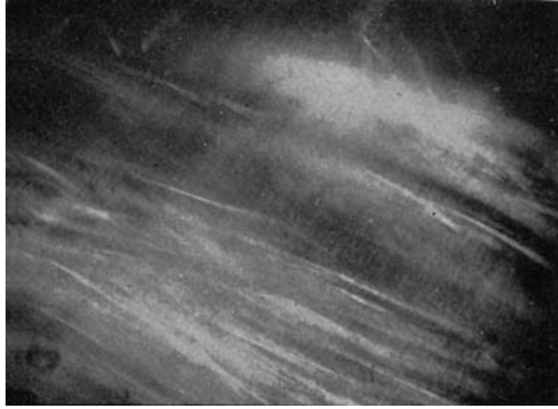
Figure 24.5 Anomalous double refraction (tabby extinction) in a synthetic spinel
