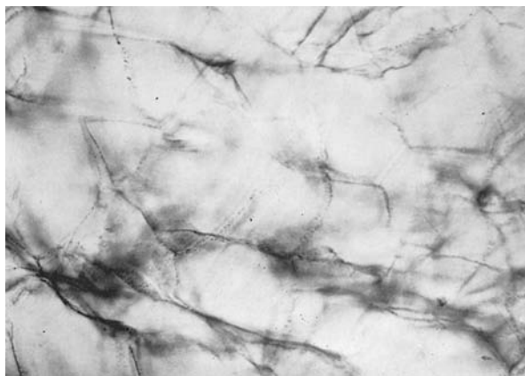
Figure 24.19 Feathers in a flux-grown synthetic emerald
