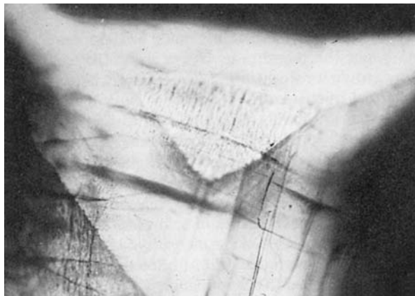
Figure 24.26 Synthetic emerald-coated beryl (Symerald) showing the reticulation of crack-like markings and one unpolished facet
