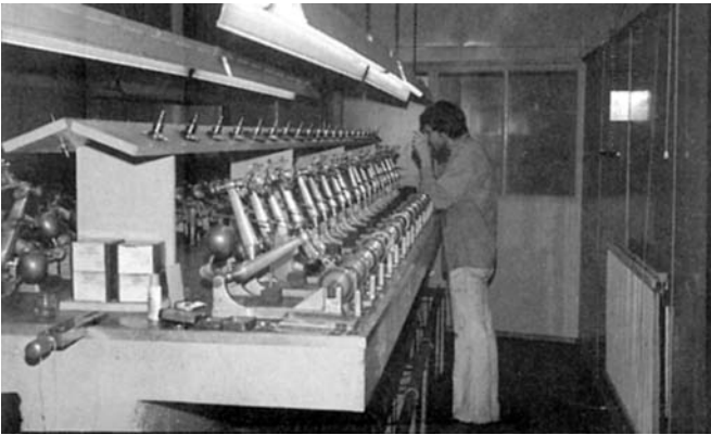
Figure 30.32 A double bank of machines attended by the diamond sawyer (courtesy of Monnikendam)
