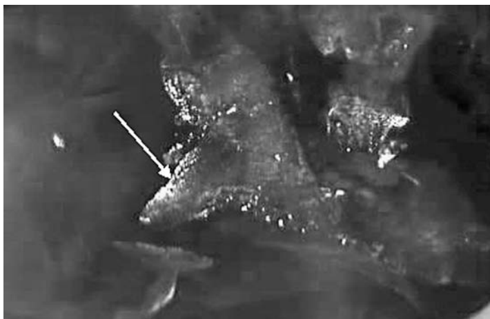
Figure 31.11 Glass-filled surface-reaching fracture (35×)
