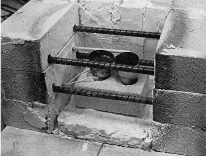
Figure 24.4 A flux-melt furnace used for the experimental production of synthetic stones (by courtesy of General Electric)
