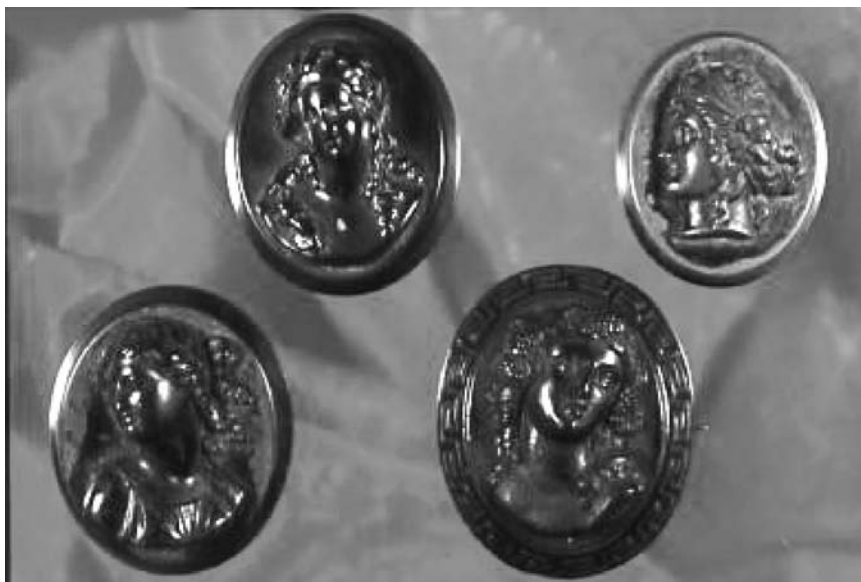
Figure 29.28 Cameos moulded from gutta-percha. Note the loss of the black paint that exposes the granular moulded surface of the underlying gutta-percha
