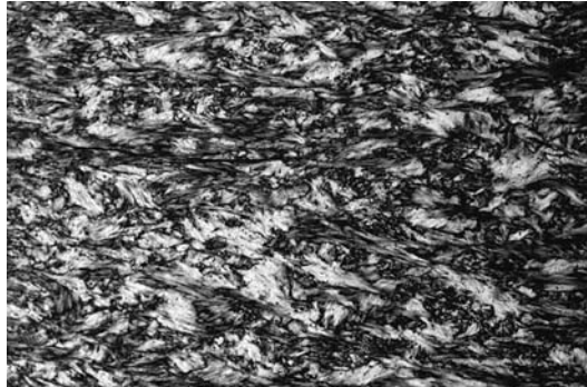
Figure 1.18 Thin section of nephrite jade from Taiwan. The variation in interference colours indicates that the fibres of amphibole vary in orientation and that they have intergrown to form a very tough rock. Field of view: 4 mm across
