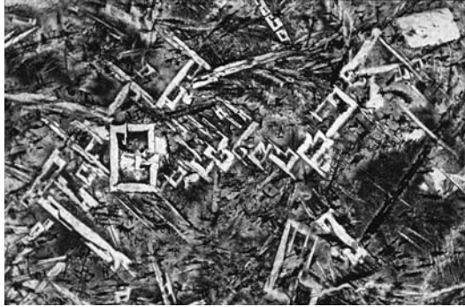
Figure 1.4 Basaltic lava containing white skeletal crystals of feldspar about 0.2 mm across in a groundmass of pale brown glass and tiny grains of magnetite. Island of Mull, Scotland
