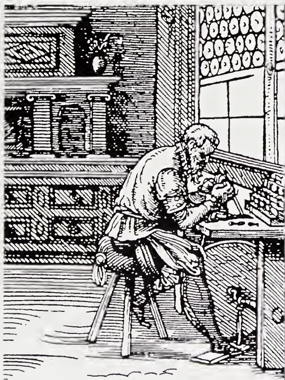
Classic stone-cutting with a foot-operated lapidary mill. Lapidarium of Jost Amman, c. 1568
