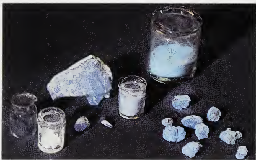
Azure (left) and azurite (right) as minerals and pulverised. In the jars on the left, lampblack and lead white.
