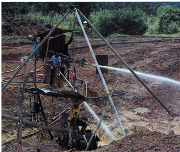
Figure 5-5. At Bo Rai, gem gravels are washed by high-pressure water cannons and transported up a pipe (seen to the right in photo) to a long sluice. Photo by Peter C. Keller.
