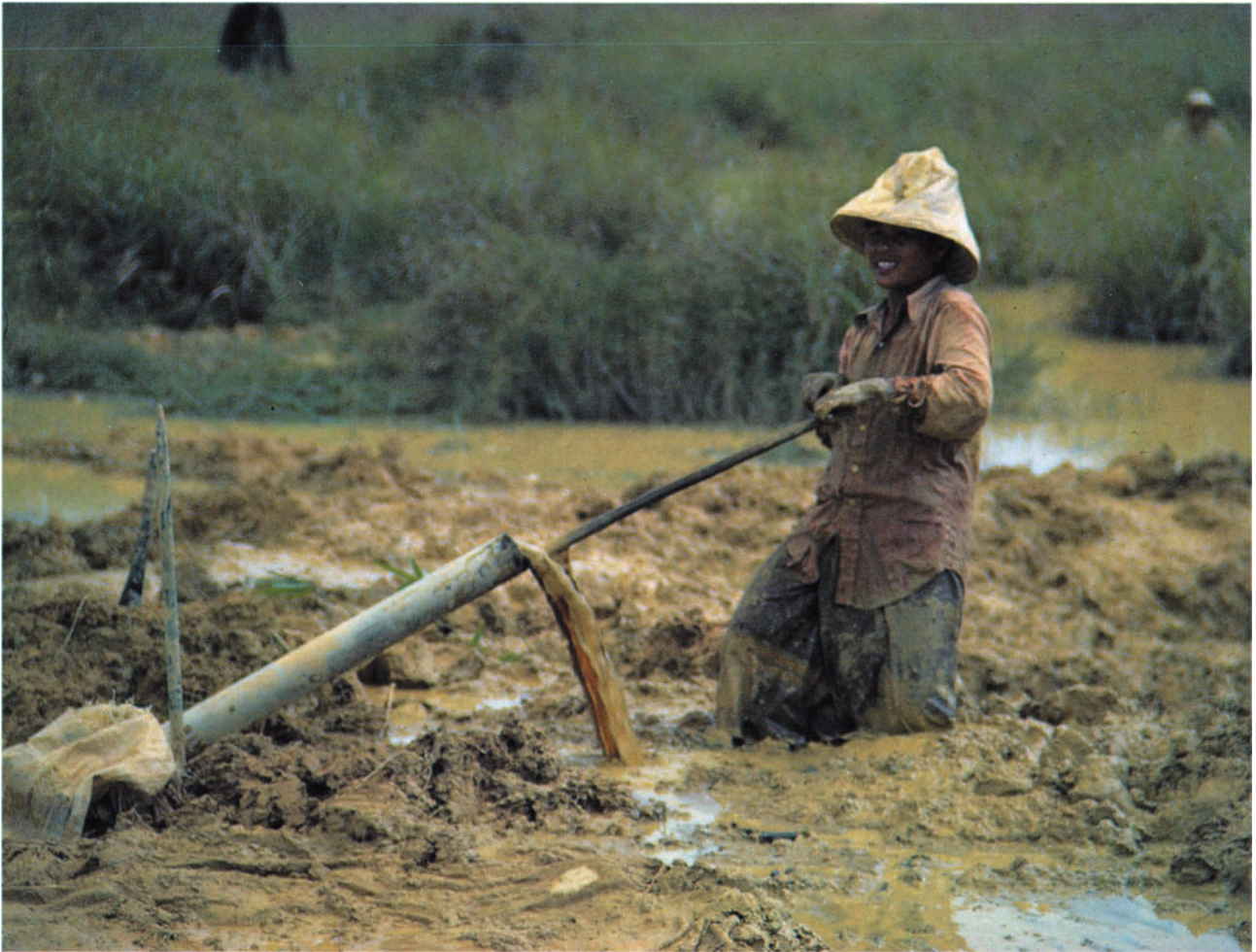
Figure 5-9. Hand pumps assist the independent miners in controlling the flooding of their workings. Photo by Peter C. Keller.
