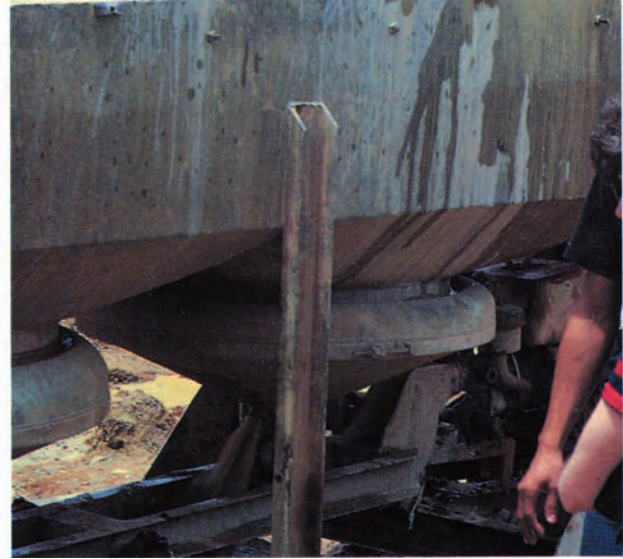
Figure 5-7. A jig or willoughby table washer, a device borrowed from the Phuket tin mines on the southern extension of Thailand, is very effective at concentrating ruby. Photo by Peter C. Keller.
