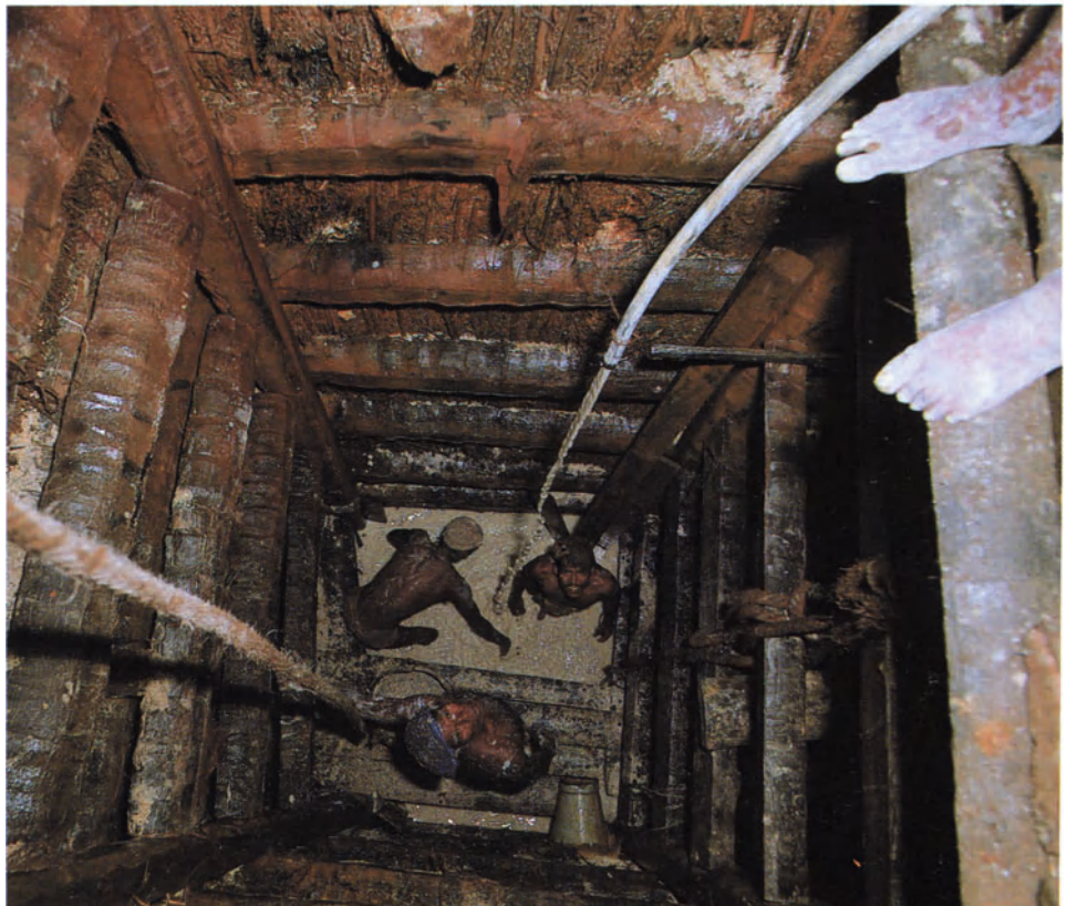
Figure 1-7. In Sri Lanka, hand-operated hoists are often used to lift buried gem gravel (known as illam) to the surface. Here, a vertical shaft has been dug through many feet of overburden to reach the illam containing sapphire, cat's-eye chrysoberyl, spinel, and many less-known gems. Photo by P. Horree.
