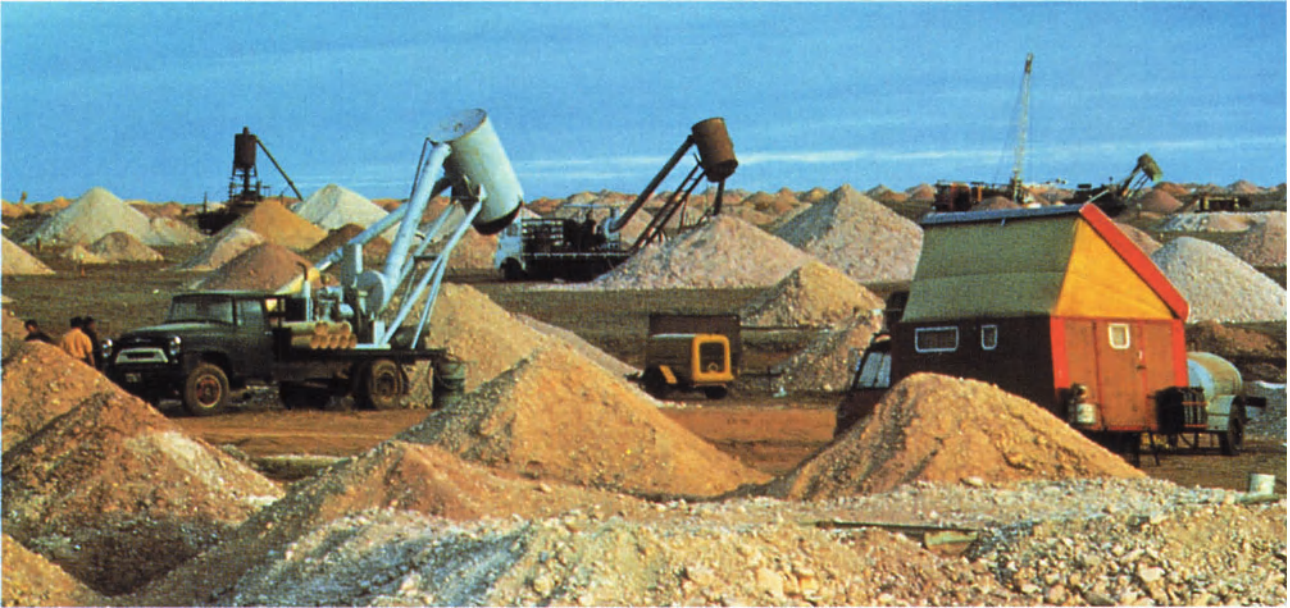
Figure 2-12. In the opal fields of Coober Pedy, South Australia, large drilling rigs or blowers bore cylindrical shafts down to the opal-bearing strata. Photo courtesy of the Department of Mines and Energy, South Australia.
