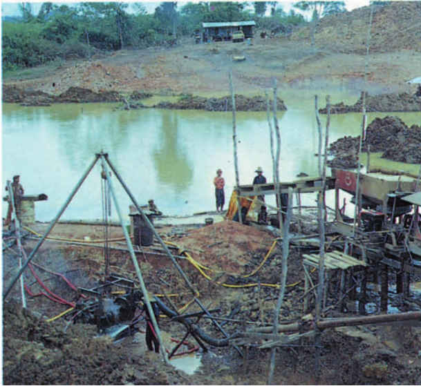
Figure 5-6. After the gem gravels exit the pipe, they are run over a long sluice. The heavier corundum concentrate collects in a jig at the end. Photo by Peter C. Keller.
