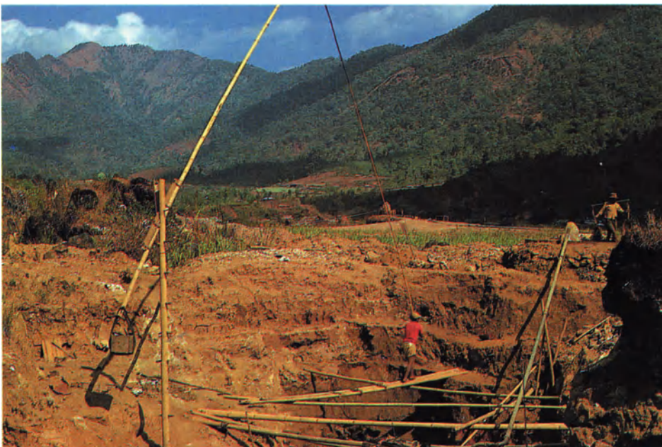
Figure 6-5. A twinlon , or circular pit, from which gem-bearing gravel is removed via the basket attached to the long bamboo crane shown here. Photo by Edward Gübelin.
