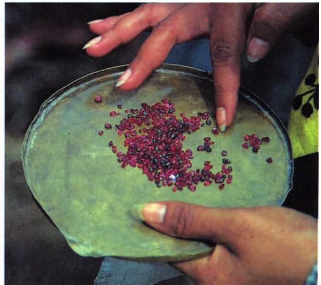
Figure 5-11. The independent miners at Bo Rai use brass trays to sort their rubies. Photo by Peter C. Keller.
