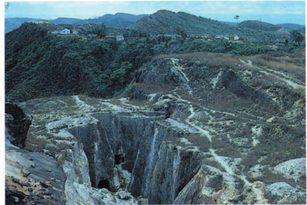
Figure 4-6. Open-pit mining at the top of the Cruzeiro mine. Note the two tunnels that follow the vein underground into the quartzite wall. Photo by Peter C. Keller.
