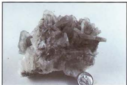
Figure 10. Light-blue, transparent to translucent, tabular barite crystals from the Mine Hills, Shirley Basin.
