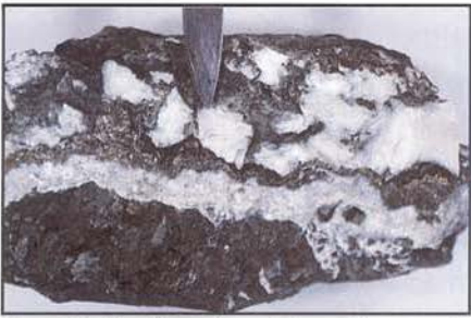
Figure 76. Massive pyrite, calcite, and quartz vein from the Snowbird mine, South Pass.
