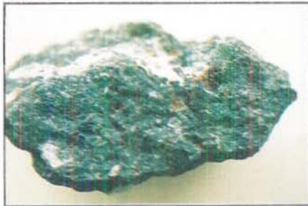
Figure 25. Kimberlite from Iron Mountain, with reddish pyrope garnet and gray, metallic picroilmenite megacryst.
