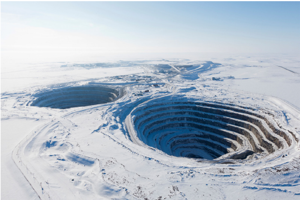
Figure 5.37 The Diavik Diamond Mine and kimberlite cluster in Lac de Gras, NWT, Canada. The open pit in the foreground is exploiting Kimberlite A154. Photo from Morley and Thompson (2006).
