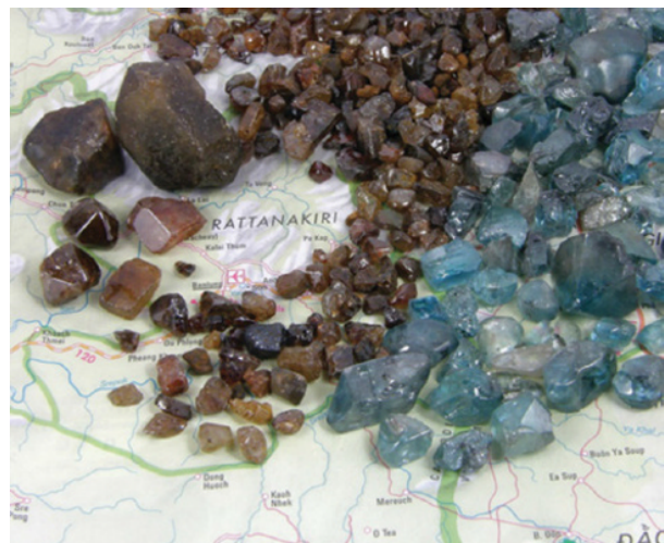
Figure 15.24 Rough zircon from Cambodia before (left) and after (right) heat treatment. Photo by P. Prachagool in Smith and Balmer (2009).
