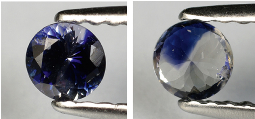
Figure 6.15 Two views of an irregularly zoned sapphire from Baffin Island, Nunavut. Note that when looking at the table of the stone the color looks well distributed, but looking through the pavilion where the light paths are different reveals how the stone is strongly zoned. The cut was designed specifically to spread the color out in order to make it look more uniform to the observer. Photo and faceting by Master Cutter Brad Wilson of Alpine Gems Ltd.
