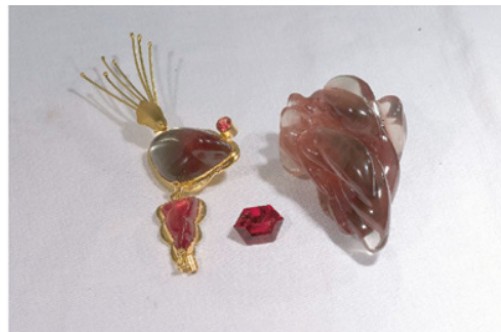
Figure 3.28 These sunstones from Oregon, USA, show varying degrees of transparency. The faceted gem in the center of the image weighs ~5 carats and is transparent. The sunstone carving on the right weighs ~175 carats and is semitransparent; it transmits light readily but the background is not transferred crisply. Smithsonian National Museum of Natural History, Department of Mineral Sciences, https://geogallery.si.edu/10002750/oregon-sunstones , photo by Ken Larsen.
