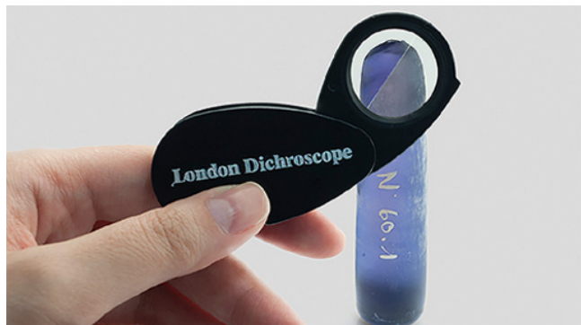
Figure 3.25 Pleochroism in a synthetic sapphire, as viewed with a polaroid-plate dichroscope. Photo by Hughes (2014).
