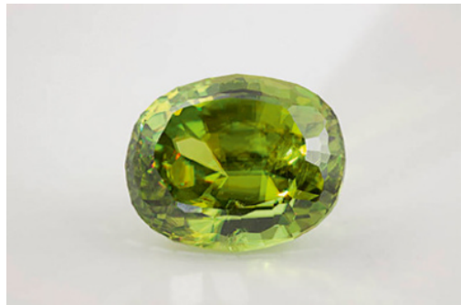
Figure 3.19 Titanite is a rare gem mineral (but common mineral) that has a high birefringence ( \Delta n = \sim 0.105 ) and in this photo doubling of the gem's rear facets is visible. This optical effect in a gemstone indicates the gemstone is anisotropic. Specimen from Madagascar and weighs 43.52 ct. Smithsonian National Museum of Natural History, Department of Mineral Sciences, https://geogallery.si.edu/10002869/titanite , photo by Ken Larsen.
