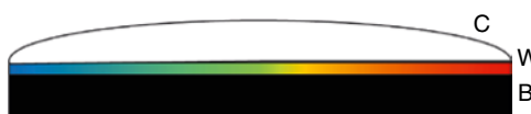
Figure 16.8 Example of a “triplet” composite gemstone: (B)acking of dark opaque material, (W)afer of ammolite, (C)ap of durable and transparent material, often quartz.
