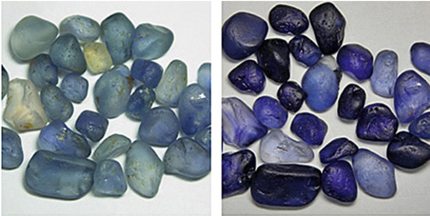
Figure 6.17 An example parcel of “before” (left) and “after” (right) heat treatment of rough sapphire. www.thenaturalsapphirecompany.com .
