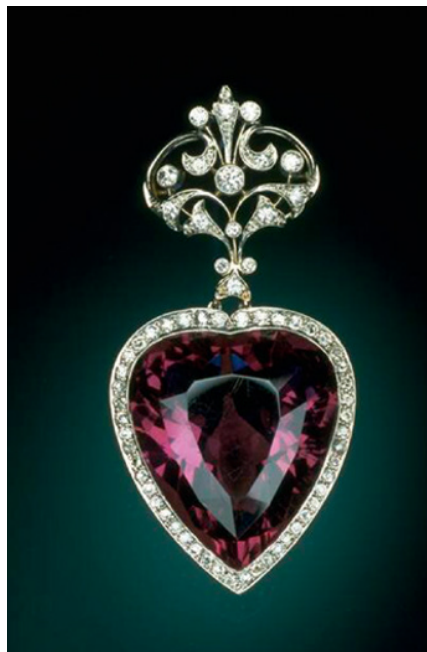
Figure 14.8 This amethyst pendant (~96 carats) shows excellent color. However, it reveals that stones with hardness as high as 7 on the Mohs scale are subject to wear; note the scratches on the table surface of this heart-shaped gem, as well as the rounding at facet joins. Smithsonian National Museum of Natural History, Department of Mineral Sciences, https://geogallery.si.edu/10002703/amethyst-heart-brooch , photo by Chip Clark.
