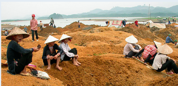
Figure B6.2.2 Rudimentary yet effective mine workings pepper the landscape. Small excavations are typically owned by an individual or family and water hoses are often seen running from nearby water sources to supply hydraulic mining practices of alluvial deposits. Images from Van Long et al. (2013).
