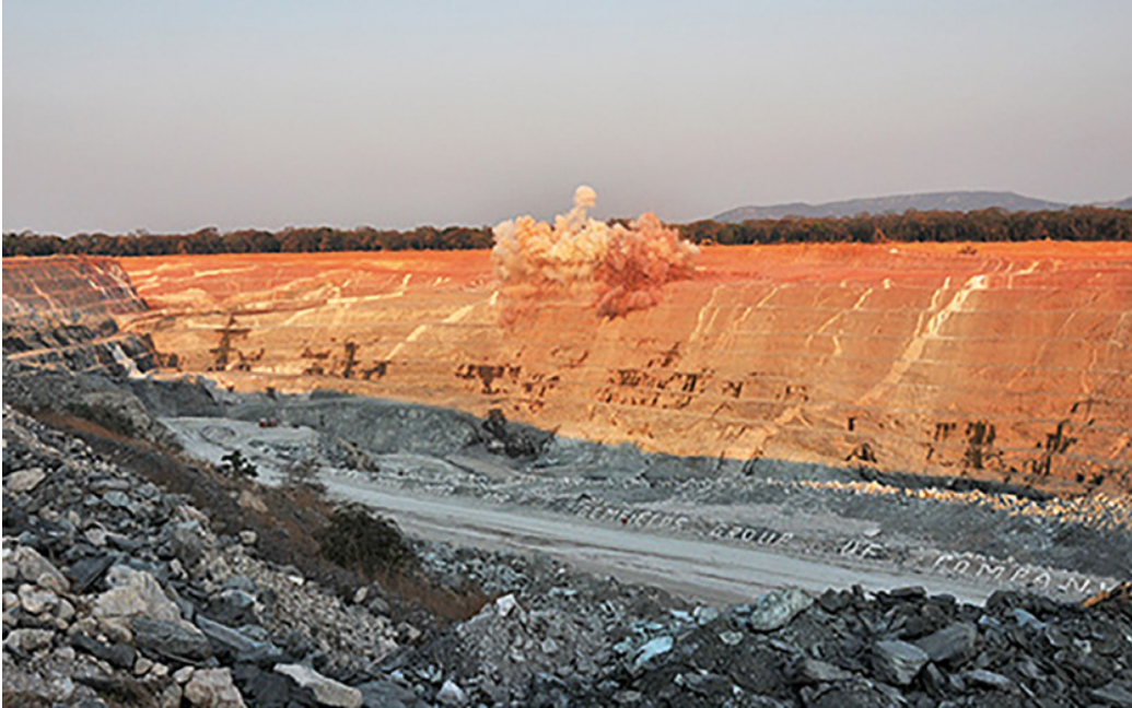
Figure 7.16 Open pit mining at the Kagem Emerald Mine in Zambia. Photo from Hsu et al. (2014) shows blasting of the pit wall where emeralds are hosted in metasomatic zones associated with pegmatites that cut amphibolite host rocks. Photo by V. Pardieu. © GIA.
