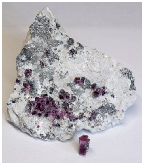
Figure 7.6 These red beryl crystals on altered rhyolite matrix are from the Wah Wah range in Utah, USA. Many of the crystals show perfect crystal form as well as color zoning. Note the flat basal termination at the top end of the loose crystal. Hand sample ~10 cm across and single crystal ~1 cm tall.
