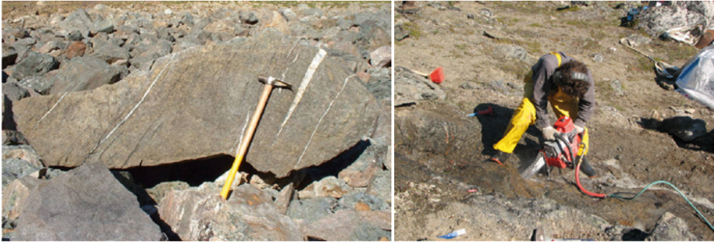
Figure 4.3 Rock hammers are necessary tools for field geology and are useful for scale in photographs – here the hammer sits next to aquamarine-bearing quartz veins (left photo). Diamond-studded chain saws are effective tools for deep and precise cuts into rock – here one is being used to sample ruby-bearing material from outcrop (right photo).
