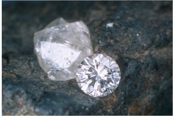
Figure 5.3 Uncut (rough) diamond octahedron (left) and cut (polished) diamond in a round brilliant shape (right) sitting on kimberlite rock. Photo by Robert Weldon. © GIA.
