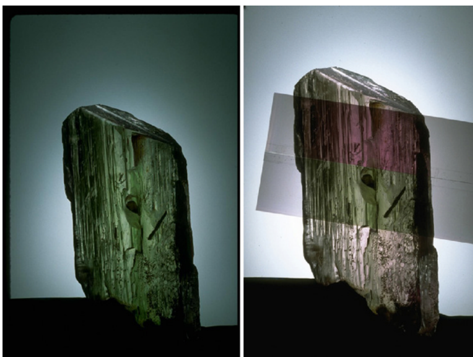
Figure 8.26 Left: spodumene in unpolarized “normal” light, as your eye would see. Right: two pieces of polarizing film between the crystal and the camera that are rotated 90° from one another. This allows both pleochroic colors to be viewed simultaneously as would be seen in a dichroscope. This particular stone is unusual because it shows both pink and green coloration. Smithsonian National Museum of Natural History, Department of Mineral Sciences, https://geogallery.si.edu/10026314/spodumene-var-kunzite , photo by Chip Clark.
