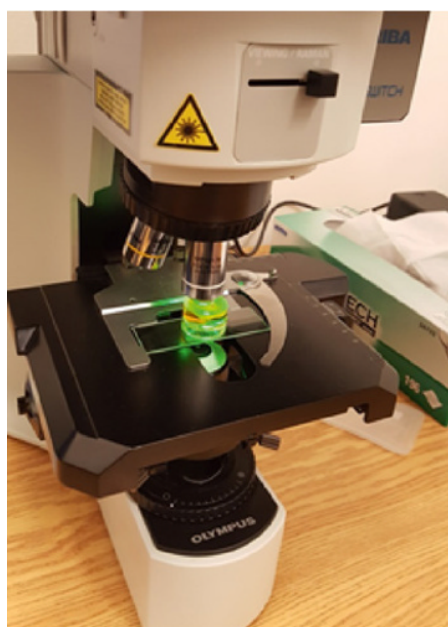
Figure 4.12 Binocular confocal microscope for nondestructive Raman spectroscopy with 532 nm green laser, visible in this photo due to scattering and refraction from the epoxy-mounted sample. Photo by D. Turner.
