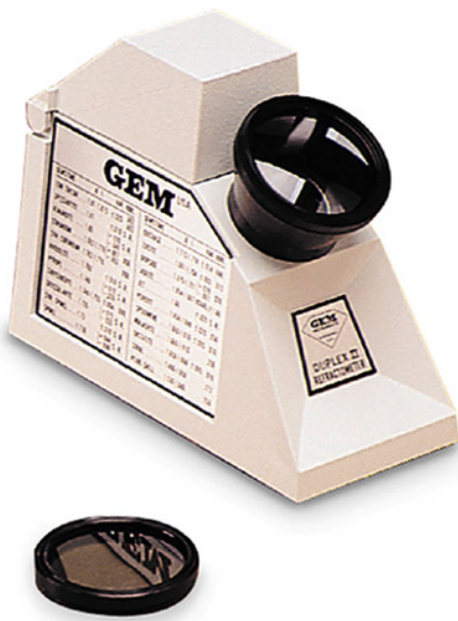
Figure 4.6 A GIA refractometer. The stone sits in a holder within the small white box. © GIA.
