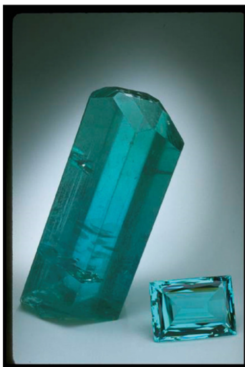
Figure 7.5 These phenomenal 15,256 carat unheated rough and 1,000 carat faceted aquamarines are from Minas Gerais in Brazil. Note the perfect hexagonal nature along the length of the rough crystal and modified basal termination at the top end of the crystal. Also of interest are the numerous fractures near the base of the crystal that are all oriented perpendicular to the c axis – these are the result of beryl's basal cleavage. The crystal also shows some vertical striations along its length. Smithsonian National Museum of Natural History, Department of Mineral Sciences, https://geogallery.si.edu/10002806/beryl-var-aquamarine , photo by Chip Clark.
