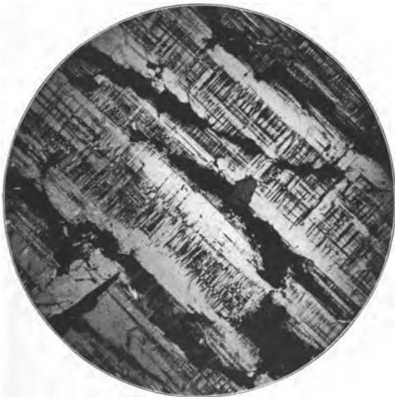
MICROPHOTOGRAPH OF THIN SECTION OF FELDSPAR FROM QUARRY OF GOLDING'S SONS COMPANY, GEORGETOWN, MAINE. MAGNIFIED ABOUT 40 DIAMETERS.
