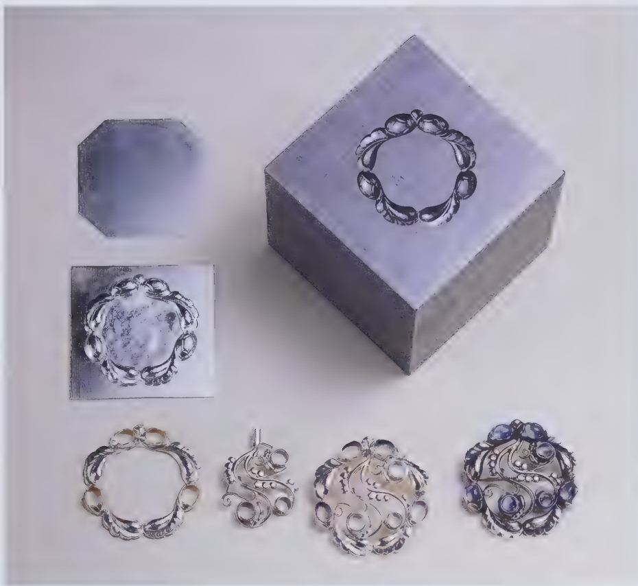
Fig. 1-27. Die punch, matrix, unfinished parts, and completed brooch GJ #159. Cast iron, silver. Collection Georg Jensen Ltd., Copenhagen. Cat. no. 226.
