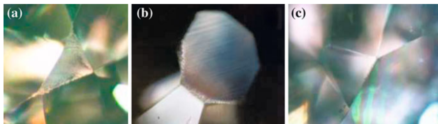
Fig. 5.6 a The facet junctions on either side of the upper girdle facets of this 0.59 ct HPHT-treated green-yellow diamond have a frosted, burned appearance, b strongly etched surface of non-repolished sites is an indicator of a high temperature HPHT treatment. Such a coarse etching is unlikely to encounter with on diamond naturals, c junctions of this small facet of an HPHT-treated diamond show traces of the frosted surface, which has not been completely removed by repolishing
