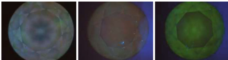
Fig. 7.7 Typical fluorescence images of natural untreated diamonds. There is no sign of enhanced fluorescence on the facet edges
