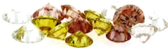
Fig. 4.6 Colorless, yellow and pink diamonds HPHT-treated by Suncrest Diamonds, USA (Simic and Zaitsev 2012)
