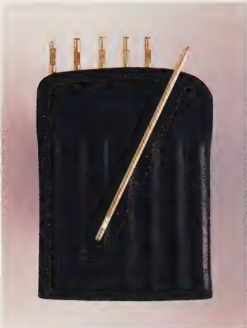
Set of scratching instruments with metal pins in which mineral splinters are set.
