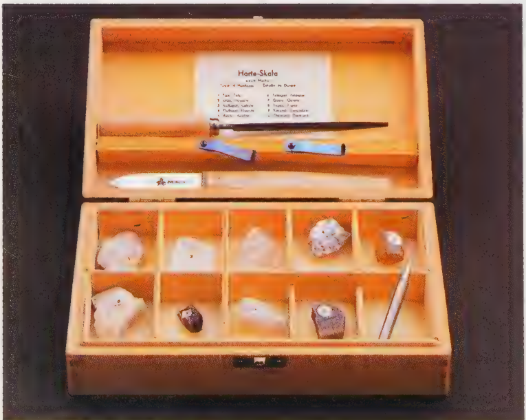
Test pieces in the Mohs' hardness scale, plus steel pin, knife and file as simple testing devices.
