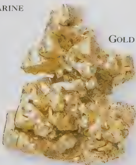
△ HACKLY FRACTURE Rough, uneven fracture surface, seen on the right of this gold specimen.
