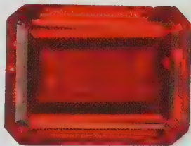
SYNTHETIC SPINEL Synthetic spinel (above), coloured red, may make a better imitation gem than flame-fusion ruby (left).
