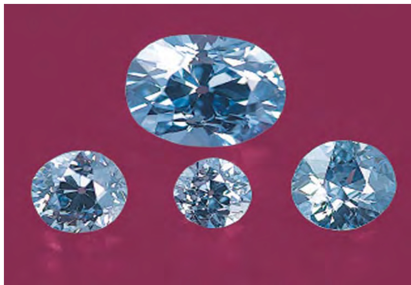
Figure 3. The four main blue diamonds are shown here removed from the necklace. The Fancy Intense blue oval at top weighs 2.60 ct, while the three Fancy grayish blue Old European brilliants weigh, from left to right, 0.75 ct, 0.42 ct, and 0.73 ct.
