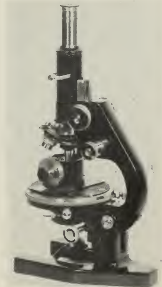
Bausch & Lomb microscope equipped with Bertrand lens and quartz wedge. ShIPLEY calibrated universal immersion stage shown in position for use.
