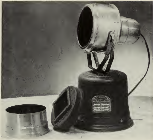
Special laboratory lamp with alternate filters for excitation of fluorescence, especially in diamonds, and for production of monochromatic yellow light for use with refractometer. ( Gemological Institute of America. )
