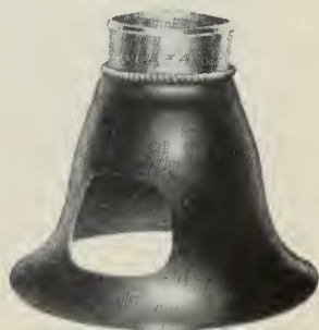
Duralumin eye loupe containing 10x triplet corrected for chromatic and spherical aberration. ( Gemological Institute of America. )
