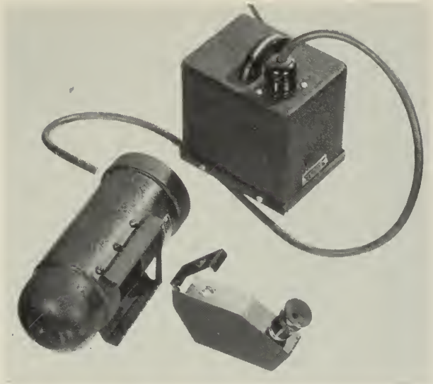
Rayner refractometer (Rayner and Keeler, Ltd.) in position for use with monochromatic lamp and transformer. Designed for use with other refractometers when lamp is in upright position. ( Gemological Institute of America. )
