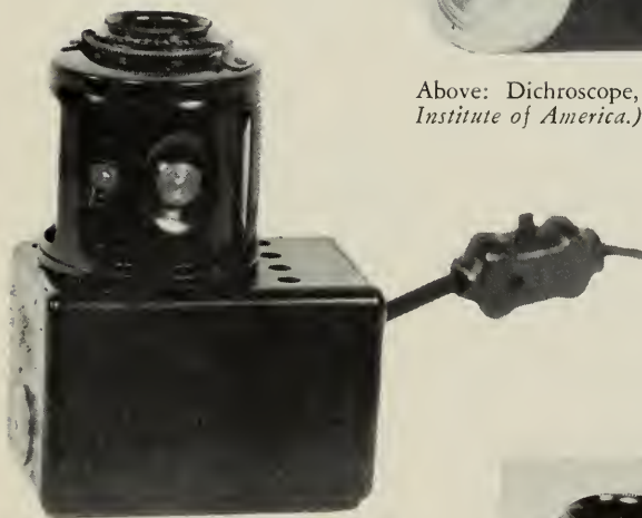
Above: Shipley polariscope on sub-stage lamp. Right: Shipley polariscope showing revolving stone holder and interior of chamber. One-half actual size. ( Gemological Institute of America. )
