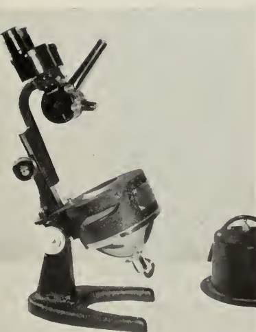
Left: Diamondscope equipped with 10\frac{1}{2}x , 22\frac{1}{2}x and 105x magnification quickly interchangeable; 105x used only for gemstone identification. ( Gemological Institute of America. )
