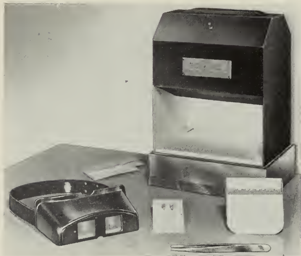
Diamolite with accessories ( Gemological Institute of America ), including 4x head magnifier ( Edroy Products Co. ), for use in grading diamonds for slight differences in body color.
