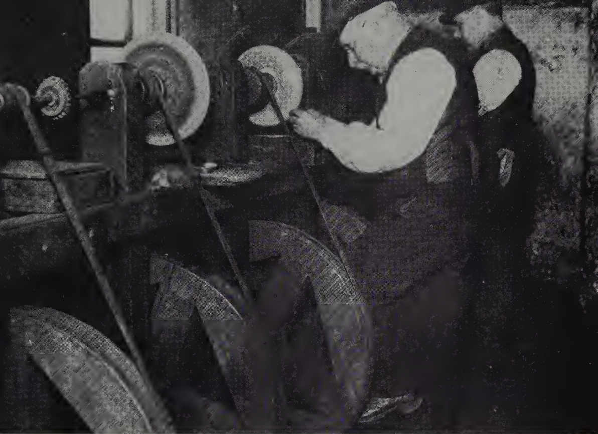
Mr J. W. Barker in his workshop with his apprentice, Joe Lyth. Mr Barker was the last man to be indentured into the jet trade and his indenture can still be seen in Whitby Museum. Mr Lyth was the last man to be apprenticed into the trade and served a full seven years apprenticeship under Mr Barker. Here they are leading. Notice the large wooden flywheels, 2 feet 6 inches (760 mm) in diameter and 4 inches (100 mm) thick, worked by a treadle, Leather straps connect the flywheel to a pulley on the driven shaft. Under the lead wheel is the box of rotten stone and on the wall are naked gas jets.
