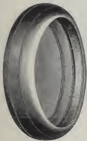
A Watch Case with folded over edges all made except putting on the Pendant and Joints.
