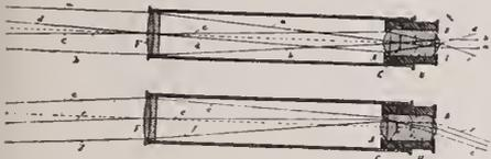
and the smaller plano-convex lens B of such proportion and relation that the image of the distant object through the object glass is formed at the center of the sphere describing the larger lens which is the focus of the smaller lens.
