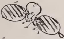
ing lower portion D<sup>2</sup>, said bends forming an off-set and the springs E rigidly attached at their lower ends to the parts D<sup>2</sup> of said nose-piece, their free ends extending upwardly substantially in the same line as the portion D<sup>2</sup> of said brackets, said upper ends being free to accommodate themselves to the nose.
