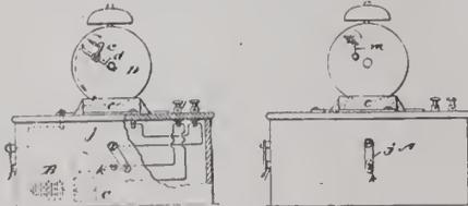
piece upon which and one of said contact plates an ordinary metallic clock is adapted to rest and an electric alarm connected with the said plates, of a circuit maker adapted to be held elevated by the winding arbor of the alarm and when released to descend upon
