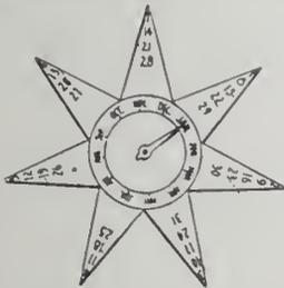
on the days of the month, and around its center, the month of the year, the star being pivotally connected with the disk at its center, and a pointer pivoted on the same pivot, the disk being provided with a loop whereby it is adapted for a watch-charm.
