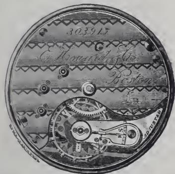
18-size, O. F., No. 7.—Adjusted to heat, cold, position and isochronism, Nickel.
