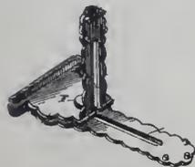
hinged together to fold face to face, and provided on their inner faces at their outer ends with series of studs G G'; one series of studs projecting into the spaces between the other, a loop E on the upper edge of the clasp and a slide movable along the clasp and holding the two members closed or permitting them to be swung apart.
