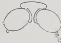
spring coil which permits the expansion of the frame for the insertion of the glass, and which automatically contracts and retains the glass firmly in the frame.
