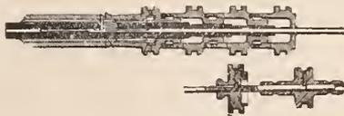
A watchmaker's tool embodying in a single organized structure a series of jewel setters of graduated sizes, means for projecting the required jewel setter into working position, an oiler housed and protected by the jewel setters, means for bringing the oiler into operative position, and a cap-jewel setter supported by and forming part of the tool structure.
