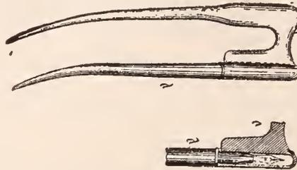
A hair-pin consisting of a head portion, a prong fixedly connected to said head portion, and a prong composed of a short socket fixedly connected to the head, and a portion detachably secured in the socket.
