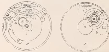
The combination of the spring barrel and shaft with the ratchet disk, mechanism for turning said shaft and disk, the spring plate 21 and connected mechanism for moving said ratchet disk to and from said spring barre', the lever 22 having the cam 25, and the curved lever or slide 27 for moving said lever 22.
