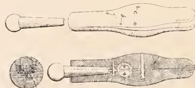
A ring clamp comprising two sections, a ring between said sections entering the same, pins passing through the sections within the ring, whereby the clamp is pivoted centrally and interiorly, and a conical pin at the rear adapted to force the jaws of the clamp together.
