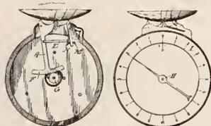
The combination in a curve measuring instrument having contact points and an indicating mechanism by which their relative positions are shown, of movable bearings by which a normal position of the object to be measured with relation to said points is secured.
