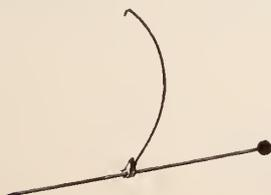
A hat pin holder comprising a flexible wire adapted to be connected at one end to the hat, and having at
