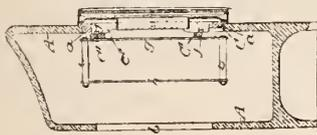
The combination of a clock case having an opening in its front, a metal ring inserted within said opening and having an external flange overlapping the margin thereof, clamping buttons applied behind said ring, and projecting within the case beyond the margin of said opening, screws for attaching said buttons to the back of said ring, a dial in front of said ring and screws for attaching the dial to said ring independently of the case.
