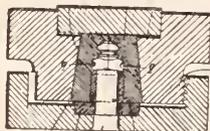
A die for making watchcase pendants that is shaped to form the same with an enlargement extending around the body portion and which comprises similar sections and a tubular part that has a cylindrical interior which conforms to the cylindrical body of the
