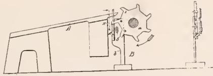
fibrous material projecting therefrom, the free and unsupported end of said fibrous material being adapted to reach contact with the side of the music tongue and damp the same.
