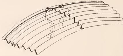
The eye-shade comprising the sectional frame, with its sections adapted to slide toward and from each other, and the sectional canopy with its sections connected to said frame sections respectively and adapted to slide one upon the other and means for connecting the shade to the nose.
