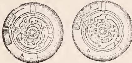
The combination in a watch, of a cover adapted to being partially rotated and having a recess, a double ended click within the recess and a ratchet wheel acted upon by one end of the click and a gear wheel therewith connected for winding the watch, a wheel adapted to be acted upon by the other end of the click and a connection therefrom to the hand setting mechanism and means for bringing one end or the other of the click into action.
