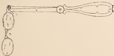
In a lorgnette the combination of a handle consisting of two levers hinged together about half way of their length, an eyeglass frame pivoted to the upper end of one of said levers, and a stud projecting laterally from said eyeglass frame, to engage with a slot in the upper end of the other lever.
