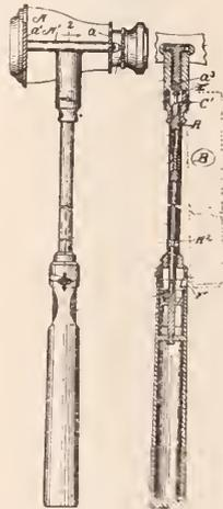
The combination of the three part holder one of such parts rigidly secured to the opera glass frame, one of the parts removably secured to the first named part, and the remaining part forming the handle adjustably secured to the second named part, with mechanism rotatably mounted in the several parts whereby the opera glass can be focused by the thumb and forefinger of the hand grasping the handle part of the holder.
