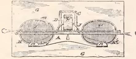
As a new article of manufacture, a spectacle-holder consisting of the plate A, having a pair of upturned-sockets B, B'; an upper, central portion C, inclining forward; a slot D, near the sides and top of said inclined portion C; and an integral-tongue E projecting from the plate A, the upper end of said tongue being free, to enable the detachment of the spectacles by lifting them bodily upward.
