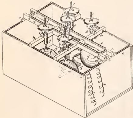
The combination of a tank, an electrolyte therein, a conducting strip mounted on the top edge thereof, a cross-tie provided with a metallic conductor directly contacting with the conductor on the tank, a movable conducting hanger mounted thereon arranged with a part in contact with the conductor on the cross-tie, an
