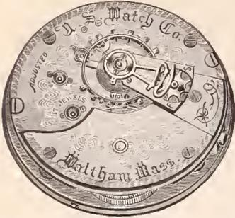
No. 80. Fine Nickel Movement, 17 Ruby Jewels in Gold settings, Safety Pinion, Hardened and Tempered Breguet Hair-Spring, Compensation Balance, Adjusted to heat, cold and positions; Patent Regulator, Double Sunk Dial.
