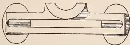
HOOKS FOR SOFT SOLDERING.
