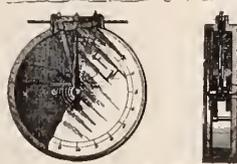
The combination in a lens measuring instrument of two sets of contact points arranged to simultaneously engage with the surface to be measured, whose relative positions are indicated by mechanism connected to the dial and to the pointer respectively.
