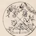
A changeable pattern plate for use in watch case designing and the like, composed of sections, each having a design portion thereon forming a part of the unitary design, said sections with their design portions being constructed and designed to fit each other and produce a complete and perfect design for all the changes or adjustments of the sections.
