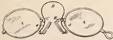
An eyeglass or spectacle provided with nose pieces extensible in planes perpendicular to the plane of the lenses, each of which consists of a strip of metal, one end of which is connected to the frame, the other end of which carries a piece of facing material for contact with the nose of the wearer, and the intermediate portion of which is bent to form a coil the axis of which is perpendicular to the plane of the lenses.
