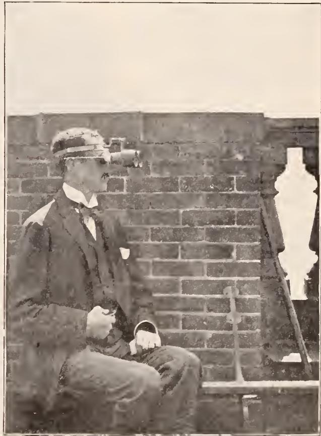
FRAME FOR HOLDING FIELD GLASSES TO HEAD. CONSTRUCTED BY THEO. MUNDORFF.
