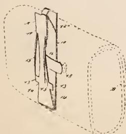
A device for securing pocket books or other articles in a pocket, the same consisting of a strip of metal
