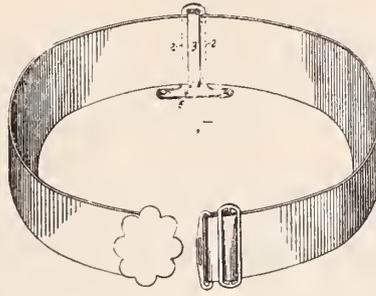
A belt slide, consisting of a rigid base plate 2, and an elastic plate, 3 joined at one end to the base plate and having at its opposite end a catch which springs into and out of engagement with a part of the base plate, said plates being arranged relatively to each other to receive between them a belt, and said elastic plate being adapted to be opened by disengaging its catch from the rigid base plate.
