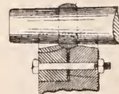
The herein described improvement in the manufacture of finger rings consisting in cutting out a circular imperforate blank, stamping the same up into a cup shape, cutting out the bottom of the cup and thereby forming a cylindrical ring blank, and swaging such ring blank between a mandrel and dies with recessed surfaces to give the blank the required sectional shape.
