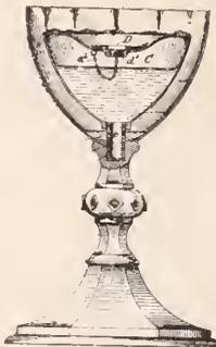
A chalice consisting of a cup-section, and a reservoir-section located in the cup-section having a discharge and vent opening at or near its base, a fill-opening in its top, and a sealing-enclosure for the fill-opening.
