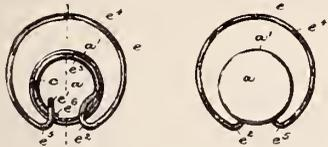
A shell or casing, having an inwardly projecting marginal rim or bead *a'* forming a chambered part in the back thereof, in combination with a bar *e* having one end bent to form a holding portion adapted to be secured in said chambered part and beneath said rim or bead *a'* of the shell or casing, and a hook on the other end of said bar.
