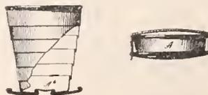
In a telescopic cup, the combination with a series of differentiated rings including a cup-like ring which is constructed with a central inwardly-extending boss, and a foot construct-
