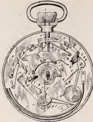
mechanism operated by one of the racks and a spring in contact with one of the arms of said lever of the first class, its free end capable of engaging the serrated face of said racks to return them to their normal position
