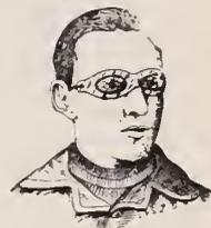
An eye-protector consisting of a transparent piece of celluloid two concavo-convex portions formed thereon adapted to fit over the eyes, flat portions surrounding said concavo-convex portions molded to conform to the shape of the face, the center portion thereof being formed into a ridge to fit over the upper part of the nose, projections formed at the ends of said protector, said projections having eyelets secured therein, an elastic cord secured through said eyelets.
