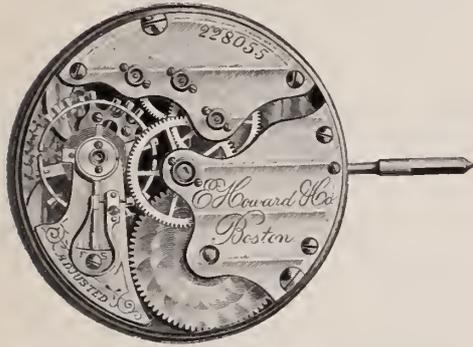
No. 8. Htg. Nickel. Divided  $\frac{3}{4}$  plate, finely damask., pat. pend. set and windg., 17 fine ruby jewels, raised gold set, hard and temp. steel barrel, comp. bal. adjg. to temp., and Isoch., pat. reg. hard. and temp. Breg. H. S., poised pal., pat. cannon pin and cen. arbor, D. S. D., roller action sight.
