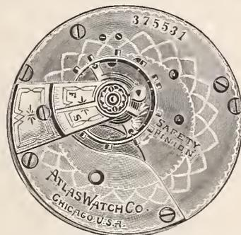
18 size, full plate, 7 jewels, nickered damaskeened, quick train stem wind and set, patent safety pinion and poised balance, hard enameled dial, double-braced mainspring, hunting lever set, open face pendant set.
