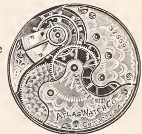
6 size, 3/4 plate, 7 jewels, nickered damaskeened, quick train, pendant set, stem wind, patent safety pinion, poised balance, hard enameled dial, double-braced mainspring, open-face or hunting.
