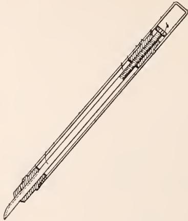
A fountain-pen comprised of a non-corrodible rod, or strong wire, passing through a tube plugged at each end, and having at both ends a tapering longitudinal groove, one for the outflow of writing fluid and the other for admission of air, and means for projecting and retracting said rod to simultaneously expose greater or less portion of said grooves or wholly closing same.
