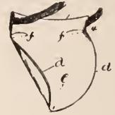
edge being bent outward to provide a relatively narrow passage or air-inlet between the shield and the face of the wearer, and the upper portions of the two side edges being bent to provide relatively narrow passages or air-outlets above the eye of the wearer.
