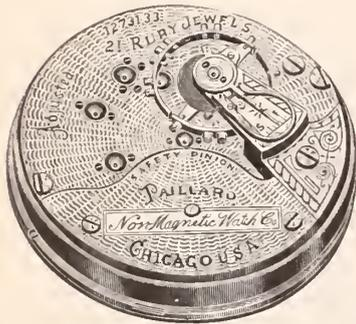
**F** Nickel, adjusted to temperature, isochronism and positions, 21 extra fine ruby jewels in gold settings, compensation balance with gold screws, patent regulator, Breguet hair-spring, double sunk glass enamel dial, elaborately damaskeened in gold with black enameled lettering.
