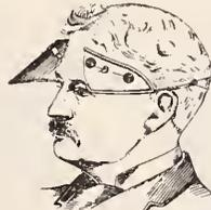
An eye-shade provided near its upper edge with a series of inwardly-projecting soft, non-absorbent pads, designed to rest against the forehead of the wearer and hold the shade from contact therewith.
