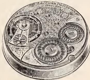
17 Ruby Jewels; Gold Settings; Jewel Pin set without Shellac; Double Roller Escapement; Exposed Pallets; Patent Micrometric Regulator; Compensation Balance in Recess, Adjusted to Temperature and Position; Patent Safety Barrel; Exposed Winding Wheels; Patent Breguet Hairspring, Hardened and Tempered in Form; Double Sunk Dial.
