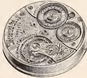
21 Ruby Jewels; Gold Settings; Jewel Pin set without Shellac; Double Roller Escapement; Exposed Pallets; Patent Micrometric Regulator; Compensation Balance in Recess, Adjusted to Temperature, Isochronism and Position; Patent Safety Barrel; Exposed Winding Wheels; Patent Breguet Hairspring, Hardened and Tempered in Form; Double Sunk Dial.
