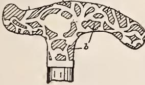
As a new article of manufacture, a rigid handle of the character described, and a sheet of flexible metal having openings therein and closely fitted to the handle, the edges of said sheet being joined together, the shape or configuration of the handle being such as to prevent the shifting of the sheet after the edges thereof are joined together.
