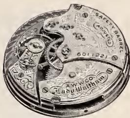
Nickel, 16 Ruby Jewels; Gold Settings; Exposed Pallets; Patent Micrometric Regulator; Compensating Balance, Adjusted to Temperature; Patent Breguet Hairspring, Hardened and Tempered in Form.
