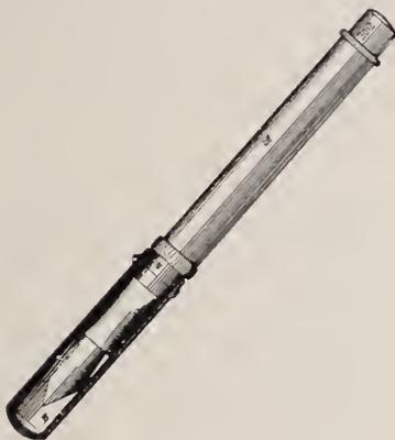
In a fountain-pen, the combination of a holder, a removable pen-protecting cap adapted to be retained in place thereon by frictional contact and supplemental means for maintaining frictional contact between said cap and holder.
