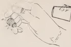
A thimble thread-cutter having a cutting portion and a clasp to embrace the thimble and composed of a helical coil whose length exceeds a circle whereby the clasp overlaps in the direction of the axis of the helix.
