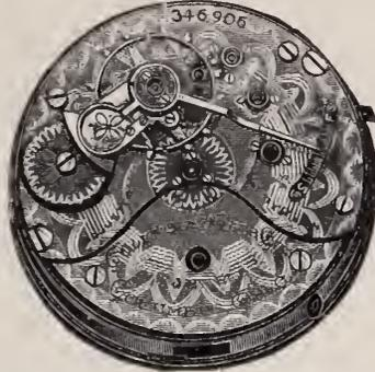
18 size, nickel, 17 ruby jewels, set in red raised gold settings, adjusted to temperature, four positions and isochronism, Breguet hairspring, patent center pinion, patent regulator, polished dust band and stem wind, pearled plates; fine white hard enameled, double sunk, red marginal figured dial; nicely damaskeened in gold on nickel.
