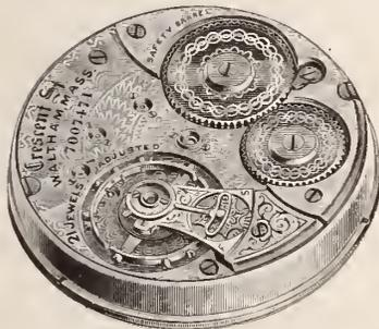
Gold Settings; Jewel Pin set without Shellac; Double Roller Escapement; Exposed Pallets; Patent Micrometric Regulator; Compensating Balance in Recess, Adjusted to Temperature, Isochronism and Five Positions; Tempered Steel Safety Barrel; Exposed Winding Wheels; Patent Breguet Hairspring, Hardened and Tempered in Form; Double Sunk Dial.
