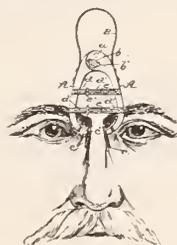
An eyeglass gage consisting of a pair of hinged caliper legs having their ends offset to a different plane from their body portions, and provided with nose clamps, and one or more gage bars located transversely on the legs between the nose clamps and the pivotal center of the legs, said gage bar consisting of two pieces, one piece attached to one leg and the other to the other leg, and the two pieces sliding telescopically over each other in the middle.
