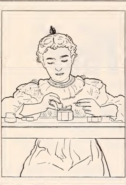
An accurately timed hairspring and balance is used as standard. The new balances to be timed are taken up, one by one, and rotated (the lower point of the staffs resting on a polished surface) until, by changing the hold of the tweezers, the new spring and the accurate standard move in perfect accord.
