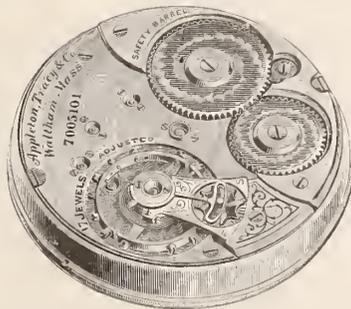
**APPLETON, TRACY & CO.**, 18 Size; Nickel; 17 Ruby Jewels; Gold Settings; Jewel Pin set without Shellac; Double Roller Escapement; Exposed Pallets; Patent Micrometric Regulator; Compensating Balance in Recess, Adjusted to Temperature and Three Positions; Tempered Steel Safety Barrel; Exposed Winding Wheels; Patent Breguet Hairspring, Hardened and Tempered in Form; Double Sunk Dial.
