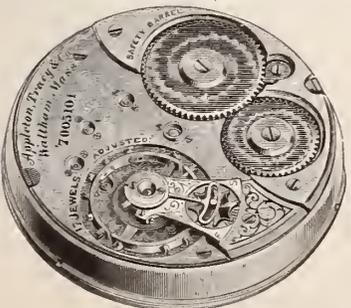
Gold Settings; Jewel Pin set without Shellac; Double Roller Escapement; Exposed Pallets; Patent Micrometric Regulator; Compensating Balance in Recess, Adjusted to Temperature and Three Positions; Tempered Steel Safety Barrel; Exposed Winding Wheels; Patent Breguet Hairspring, Hardened and Tempered in Form; Double Sunk Dial.
