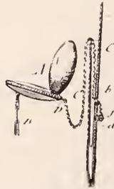
The combination, with a garment provided with a pocket, and a hole or eyelet in the rear wall of the pocket and in the lining of the garment, of a safety guard chain adapted to pass through said holes or eyelets, means for attaching said guard chain to a watch, and means for attaching the guard chain to the garment.
