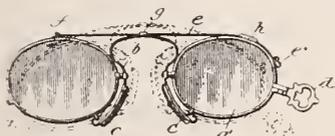
The combination with eyeglasses of ordinary construction of an adjusting band constructed of a continuous strip of material secured at one end to one of the lenses and extending over the bow to the other lens, and having a sliding connection with said bow and last mentioned lens, and terminating in a finger-piece.
