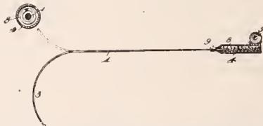
In a temple for spectacles, the combination, with a cylindrical barrel, one end of which is perforated and the other end is open of a longitudinally-movable rotatable bow portion, the inner end of
