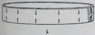
A. Showing three stages in making a molding by the first method described; 1. Circular band, showing stitches. 2. Circular band, with square wires in position. 3. The finished molding.
