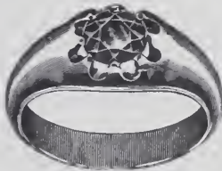
Oval Belcher ring as received with claws badly worn. Stone cannot be reset, as it would be too low to look well and the point would come below the inner circle of ring. (See cut No. 2 of flat helcher.)
