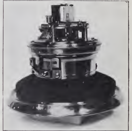
CHRONOMETER MOVEMENT MADE WITH GLASS SPRING 50 YEARS AGO.
