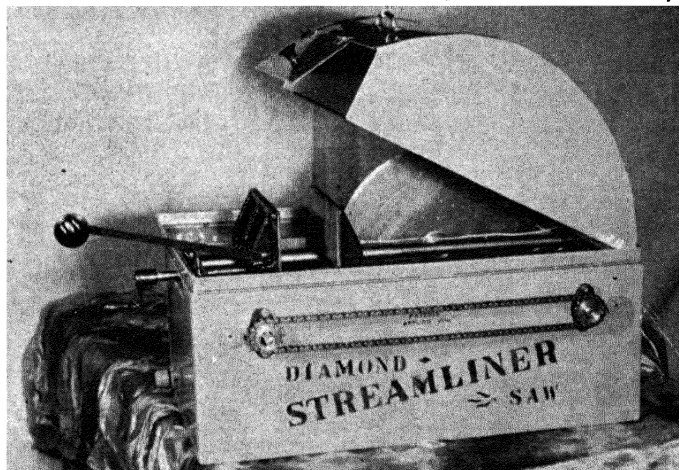
Fig. 125.—Carriage type sawing outfit. (Courtesy of W. C. Eyles, Bayfield, Colo.)
