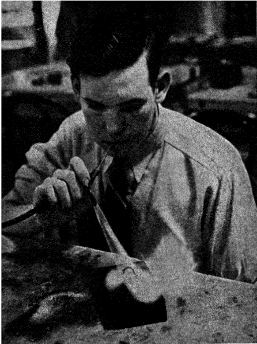
Fig. 49.—Student silver-soldering a ring, using mouth blowpipe and artificial gas.
