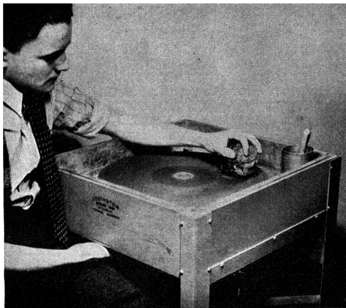
Fig. 155.—Lapping a mineral specimen on a cast-iron lap using silicon carbide grit.
