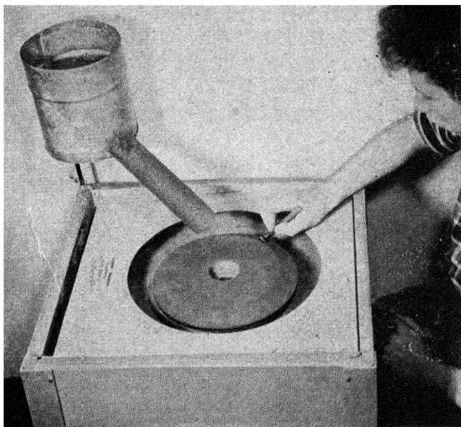
Fig. 154.—Grinding a cabochon on a plate-mounted silicon carbide wheel screwed to the vertical shaft of a lap unit.
