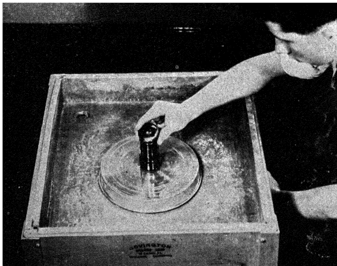
Fig. 150.—Lapping a sphere in a metal cutter mounted on a vertical spindle.
