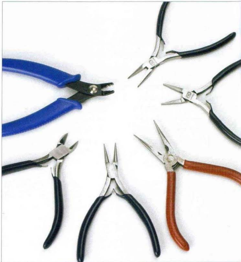
You can make all of the projects in this book with a few basic pliers and good-quality wire cutters. Clockwise from top left: crimping pliers, chain-nose pliers, flat-nose pliers, needle-nose pliers, round-nose pliers, and wire cutters.
