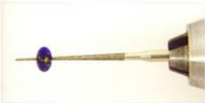
Use a bead reamer to enlarge the diameter of the bead's hole.
