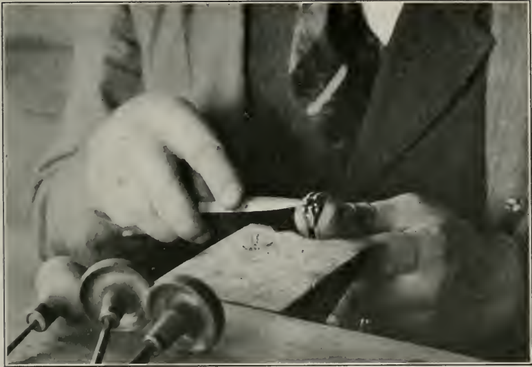
FIGURE 96. Filing the top of prongs
