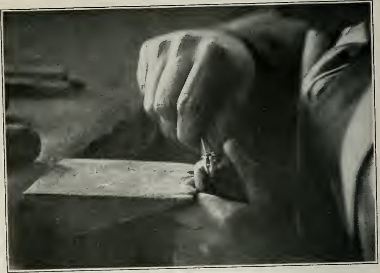
FIGURE 94. Setting the stone. First step
