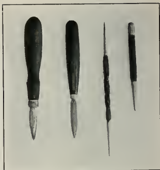
FIGURE 163 Burnisher Scraper Scratch Awl Center punch
