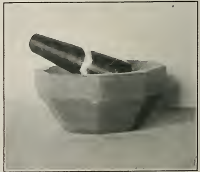
FIGURE 117 Agate Mortar and Pestle
