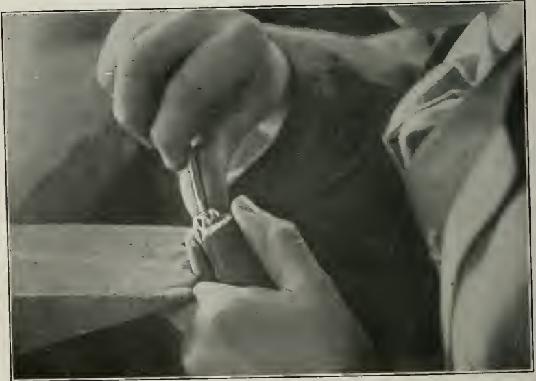
FIGURE 95. Setting the stone. Second step [158]
