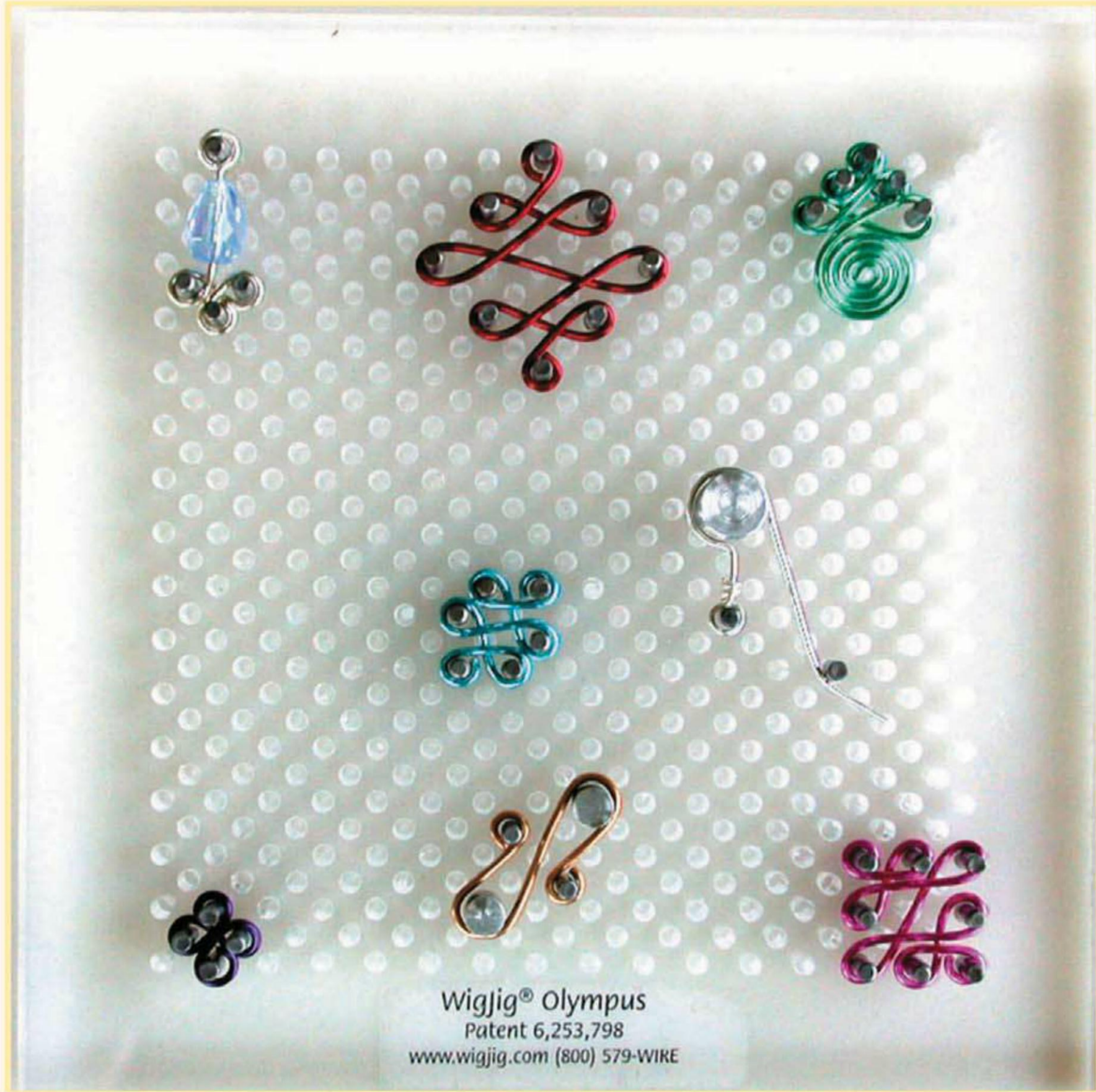
A wire jig is a possible alternative to using hand tools for making wire findings and other components.
