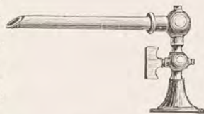
FIG. 35. Jeweller's Soldering Burner for gas.
