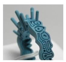
Wax Model — Before a ring is cast in precious metal, a model of it is carved in wax. Wax models are carved by hand or by a computer-assisted machine.
